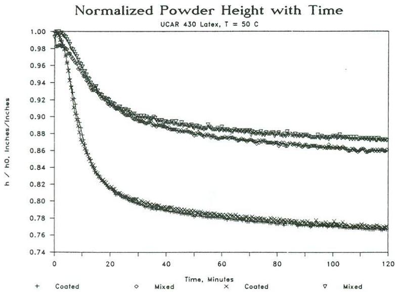
Figure 5. Sintering rates of mixed and coated alumina
