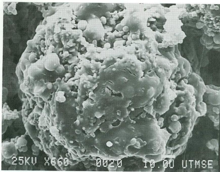
Figure 2. Alumina particle coated with UCAR 430 polymer
