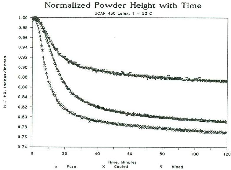
Figure 4. Sintering rates of UCAR 430 samples
