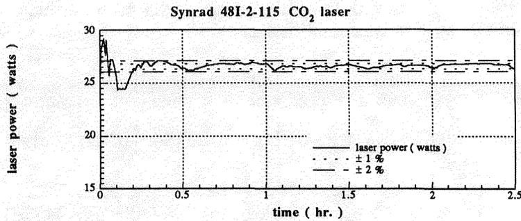
fig.5 Stability measurement of the laser power source
