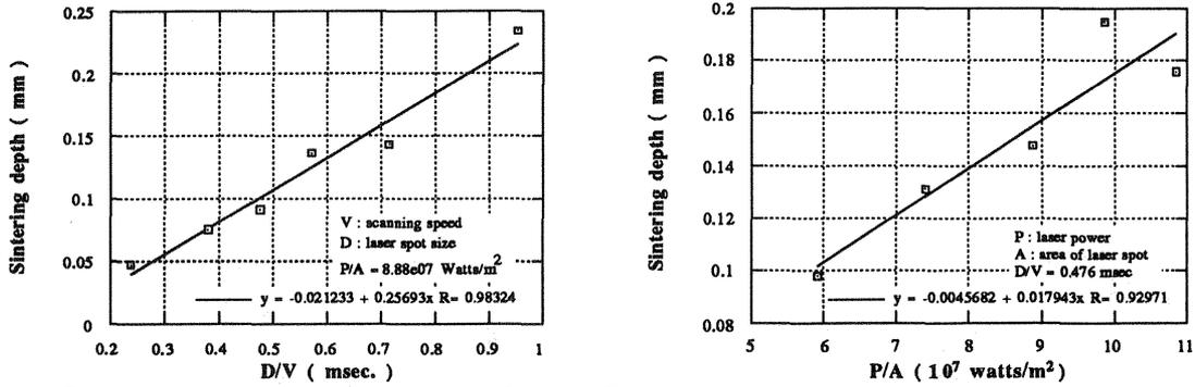
fig.8 Relation between the degree of solidification and laser power and scanning speed
