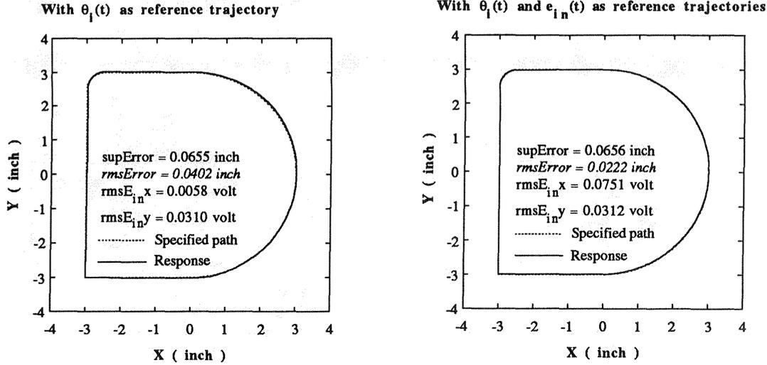
fig.14 The simulation results for both implementations
