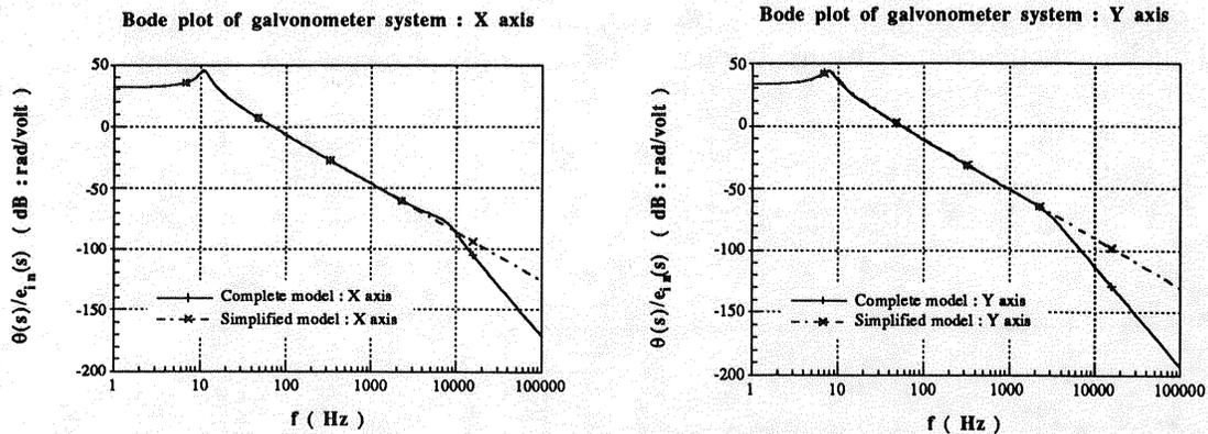
fig.4 Bode plot of complete/simplified galvanometer model
