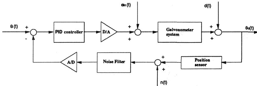
fig.13 The block diagram of control system
