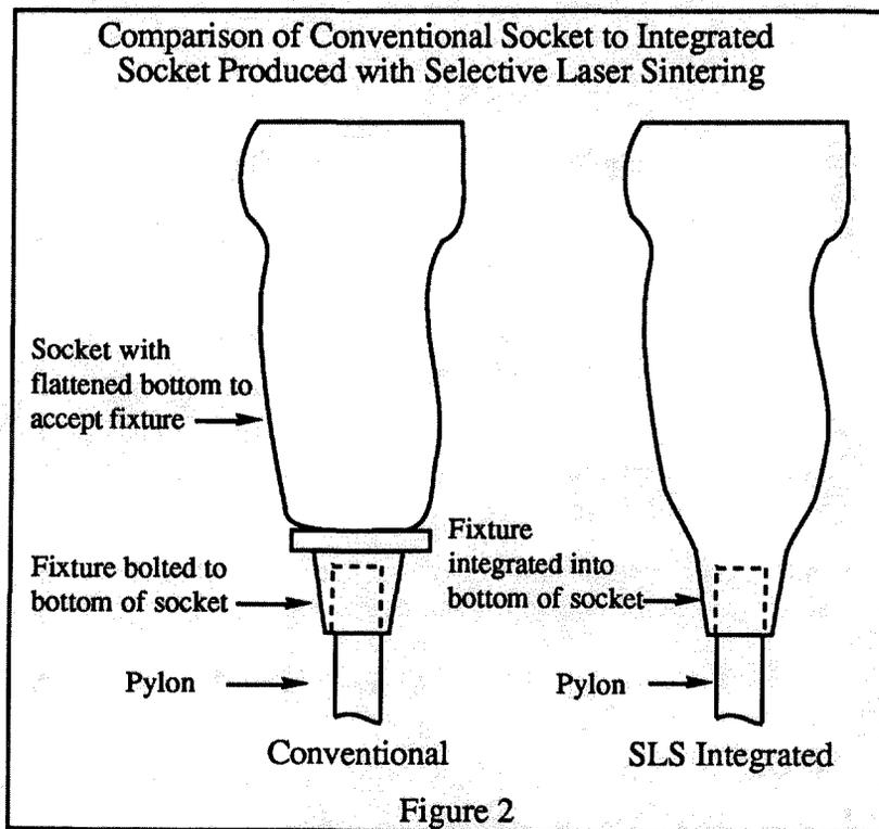
The integrated fitting is designed to accommodate a standard 30 mm pylon. A pylon location is completely reproducible as it is added during the design process rather than after socket construction. As can be seen in figure 2, the socket shape does not need to be distorted to accommodate a fitting. The integrated SLS socket preserves the anatomical shape at the distal end of the limb.
