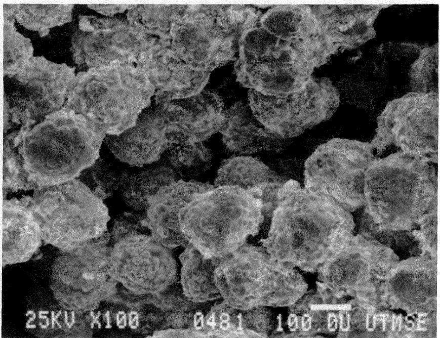
**Figure 5.** A micrograph of an annealed, multiple layer sample. The sample was annealed in H<sub>2</sub> at 800°C for 24 hrs. The laser power was 17W and the scan speed was 3.41 cm/s. The magnification is 100X.
