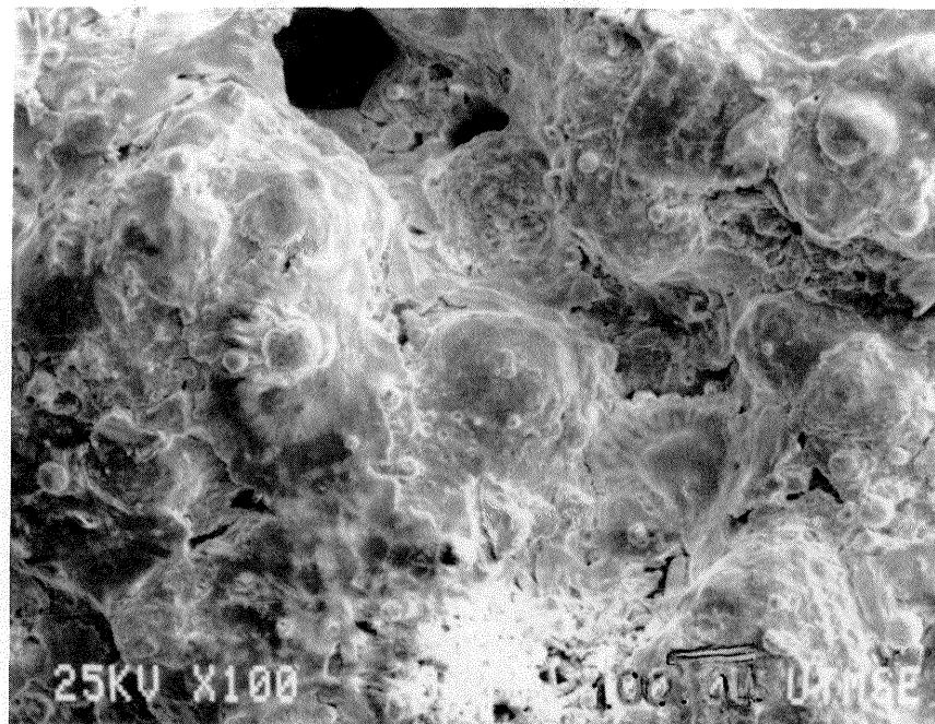
**Figure 2.** Micrograph showing the surface of an unannealed single layer sample. The laser power was 17 W and the scan speed was 3.41 cm/s. The magnification is 100X.
