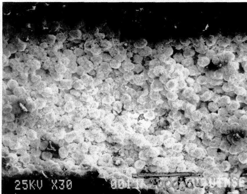
**Figure 7.** A cross section of an annealed sample (800°C for 24 hrs in H<sub>2</sub>). The layers are completely indistinguishable. The laser power was 17 W and the scan speed was 3.41 cm/s. The magnification is 30X.
