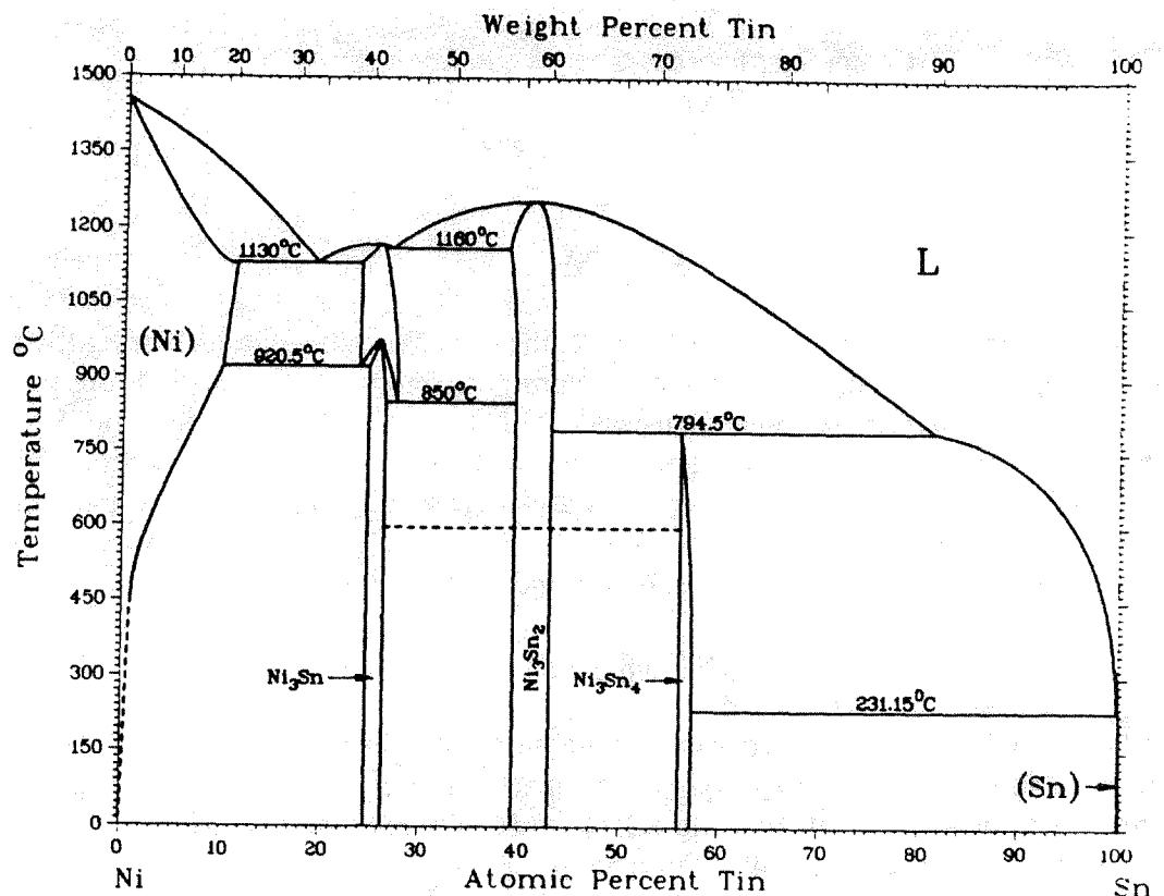
**Figure 1.** The Ni - Sn Phase Diagram. ( From Binary Alloy Phase Diagrams).
