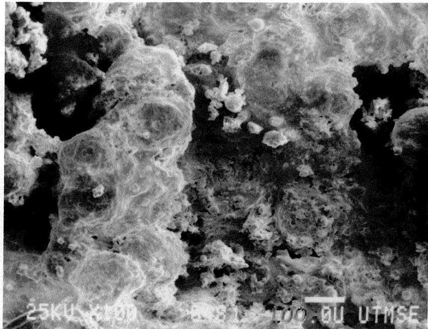
**Figure 4.** A micrograph showing the surface of an unannealed, multiple layer sample. The laser power was 17 W and the scan speed was 3.41 cm/s. The magnification is 100X.
