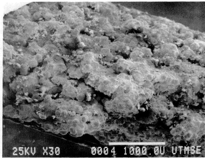
**Figure 6.** A micrograph showing a cross section of an unannealed, multiple layer sample. The layers are barely distinguishable. The laser power was 17 W and the scan speed was 3.41 cm/s. The magnification is 30X.
