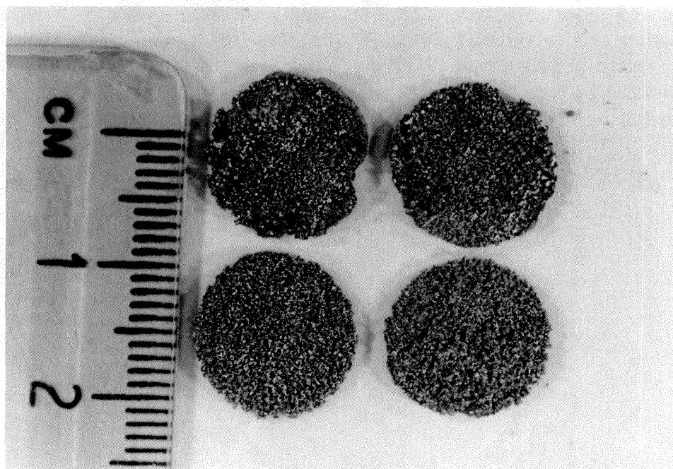
**Figure 3.** Single layer samples showing the influence of laser parameters. The top samples had a laser power of 25 W; the bottom samples had a laser power of 17 W. The left side had a scan speed of 4.55 cm/s; the right side had a scan speed of 3.41 cm/s.
