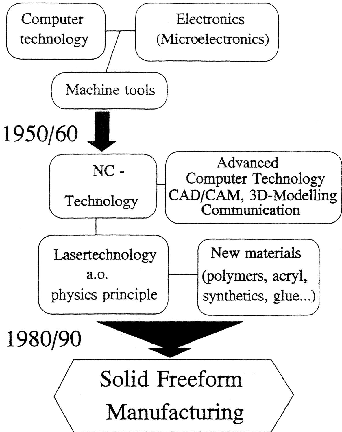
**FIG 2: Developmental steps in advanced manufacturing technology**
