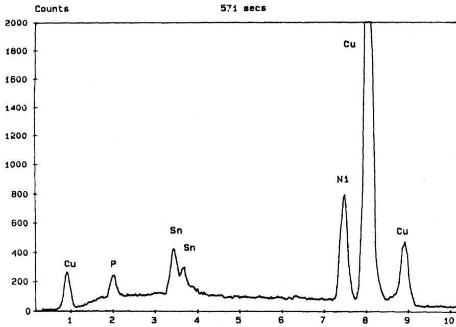
Figure 7 EDS analysis of SLS sintered 60 wt% Bronze-30 wt% Ni -Cu<sub>3</sub>P.
