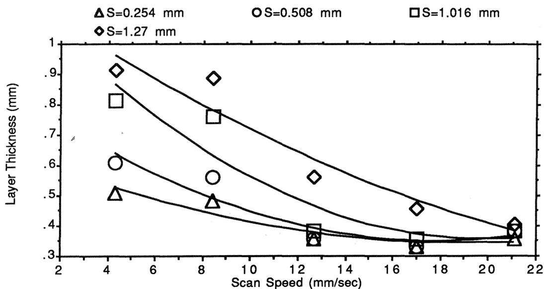
**Figure 2** SLS sintering layer thickness as a function of laser scan speeds and scan line spacing. Laser power = 200w, beam size=4.5 mm, nitrogen flow rate = 60 l/min, no powder bed biasing temperature, for copper powder ( $\sim 100\mu\text{m}$ ) material.
