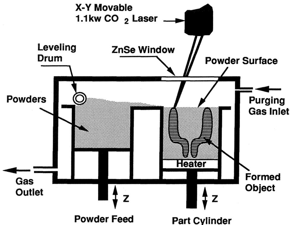
Figure 1 Sintering cell for high laser power SLS
