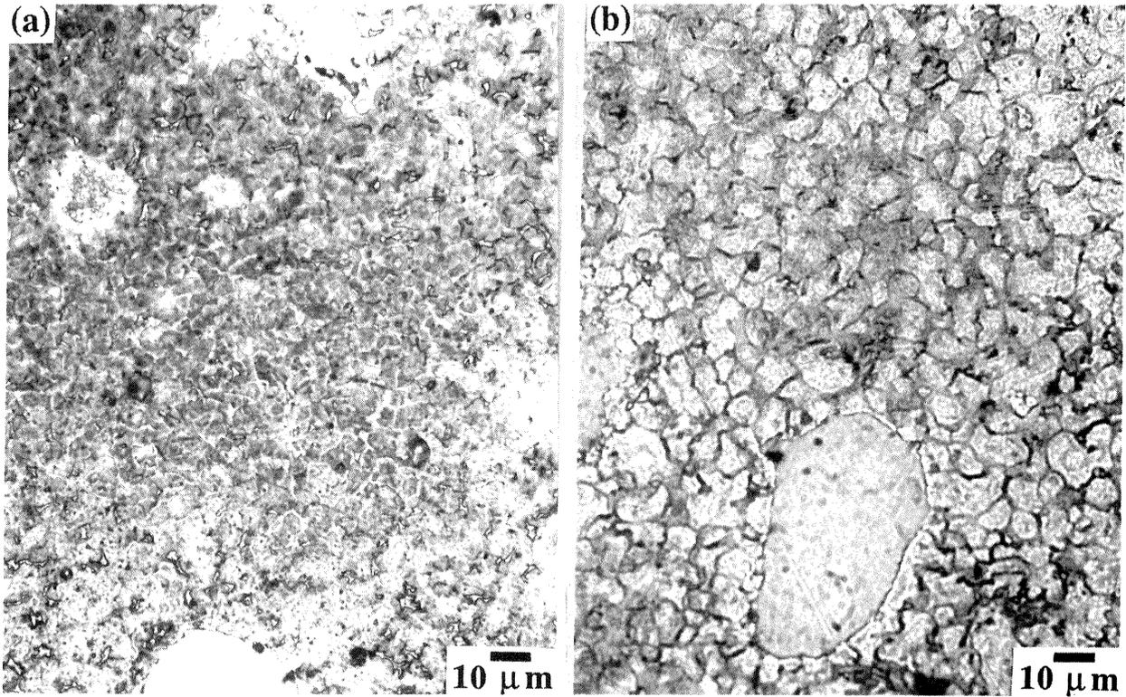
**Figure 4** Microstructure of Bronze+Ni+Cu<sub>3</sub>P sintered at laser beam size=4.5 mm, scan speed = 21.2mm/sec, scan line spacing =0.5mm, purging nitrogen flow rate= 60 l /min, no powder bed biasing temperature, and (a) laser power = 200w, (b) laser power = 280w.
