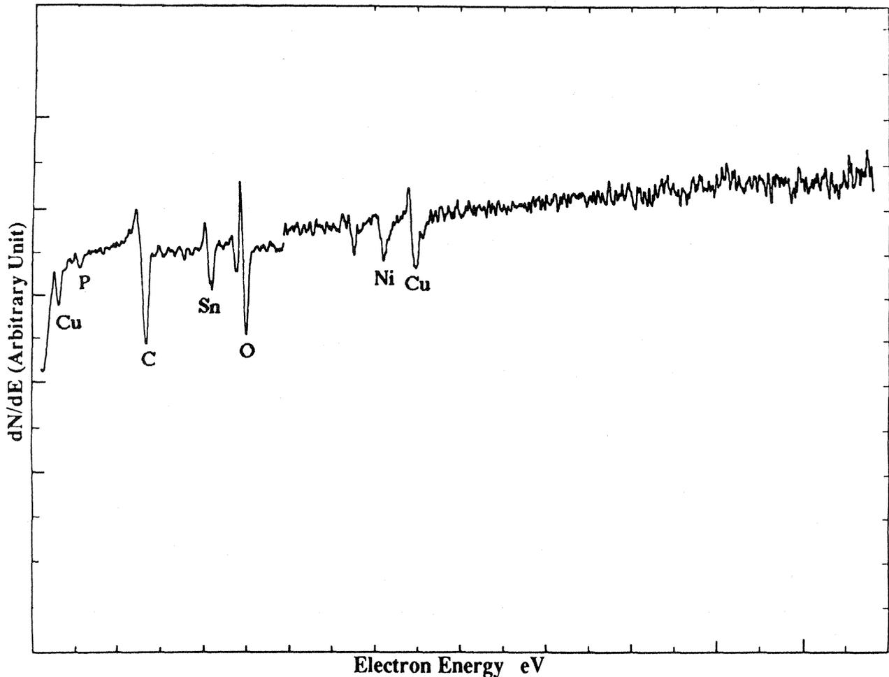
Figure 10 AES analysis of the in-situ fracture surface of the SLS sintered 60 wt% Bronze-30 wt% Ni -Cu<sub>3</sub>P.
