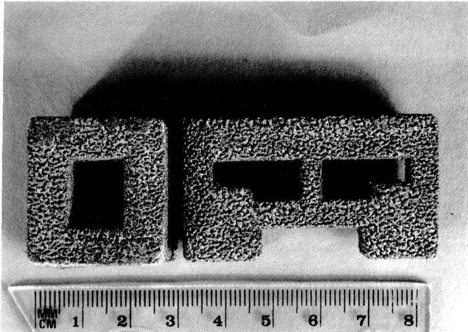
Figure 11 SLS fabricated WC-Co-Ni parts.
