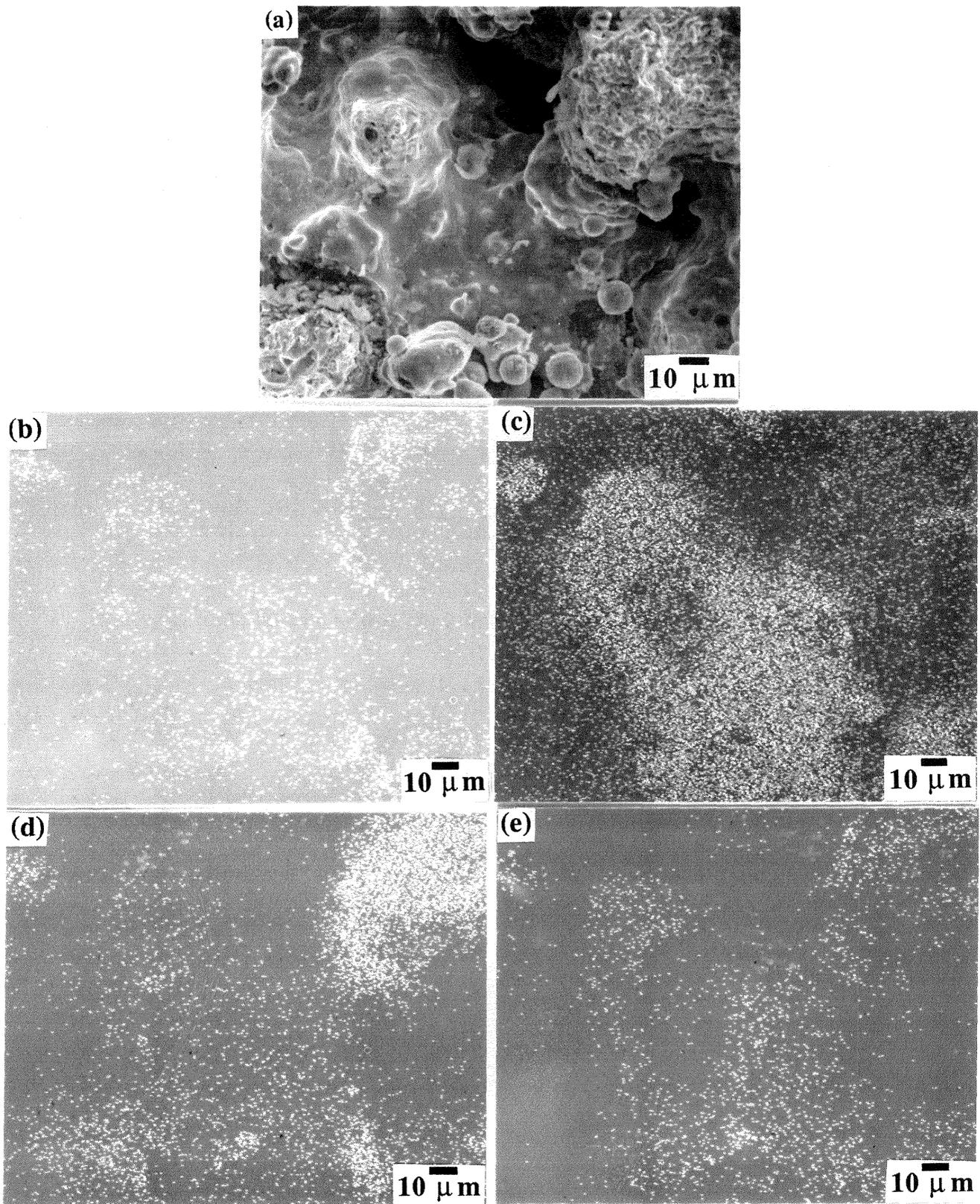
Figure 9 The secondary electron image (a) and X-ray element maps of (b) P, (c) Cu, (d) Sn, and (e) Ni from the fracture surface of the SLS sintered 60 wt% Bronze-30 wt% Ni -Cu<sub>3</sub>P.
