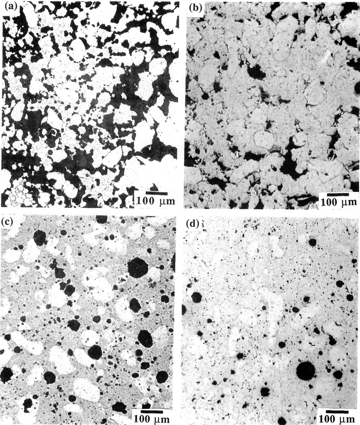
**Figure 3** Microstructure of Bronze+Ni+Cu<sub>3</sub>P sintered at laser beam size=4.5 mm, scan line spacing =0.5mm, purging nitrogen flow rate= 60 l /min, no powder bed biasing temperature, and (a) laser power = 200w, scan speed = 21.2mm/sec, (b) laser power = 200w, scan speed = 12.7mm/sec, (c) laser power = 280w, scan speed = 21.2mm/sec, (d) laser power = 280w, scan speed = 12.7mm/sec.
