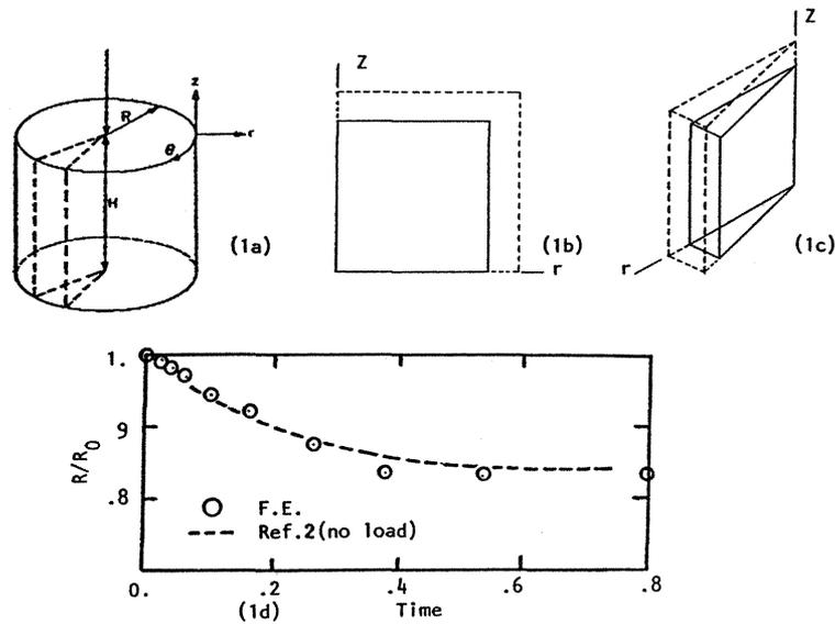
Fig. (1a) Solid Cylinder (Ref.[2]), (1b) Deformed Cylinder (4-node model), (1c) Deformed Cylinder (8-node model), (1d) Radial Reduction vs. Time
