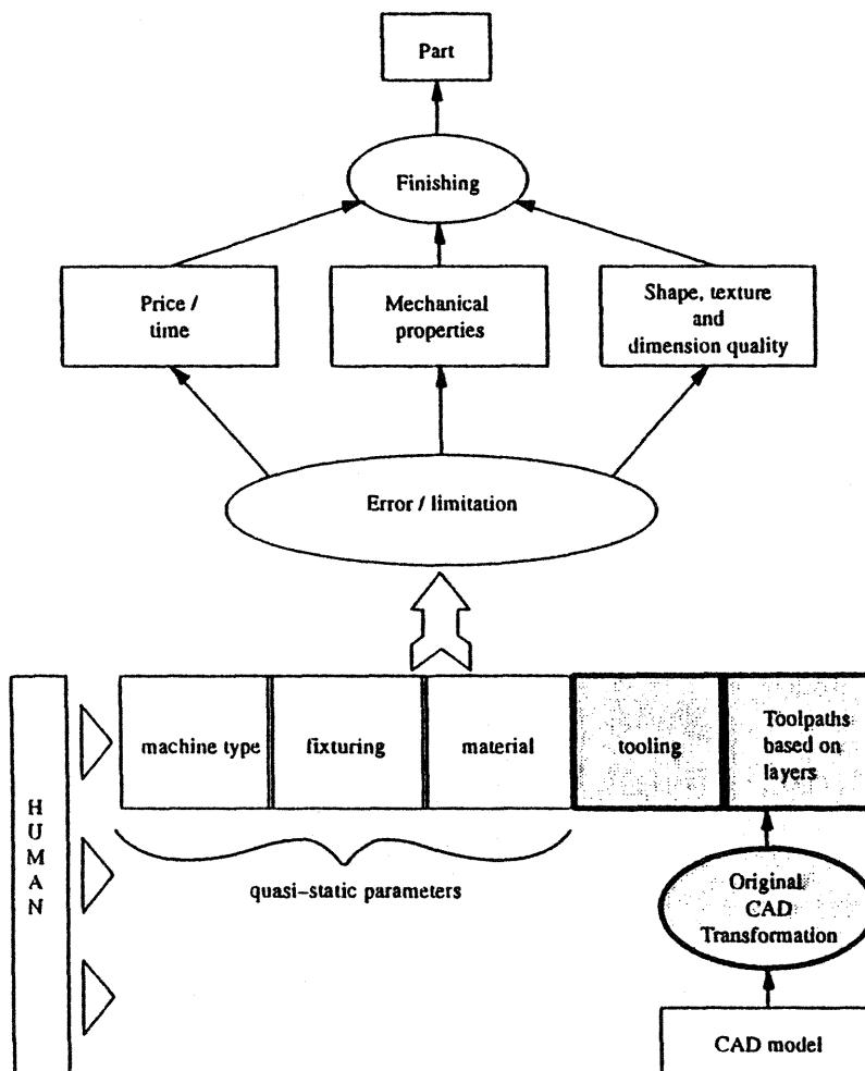
**Figure 3:** Adaptive Laminated Machining: Environment and Goals
