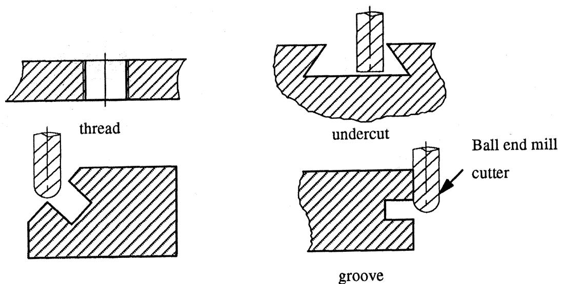
**Figure 7:** Examples of geometrical constraints in adaptive laminated machining
