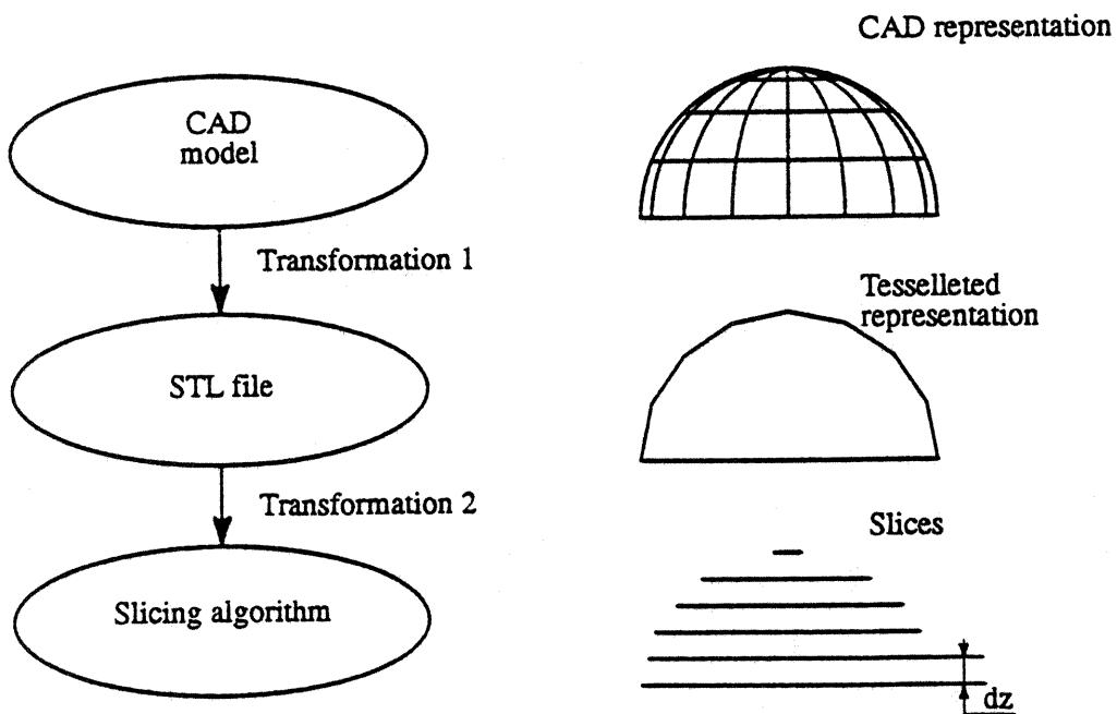
**Figure 2:** Slicing Procedure
