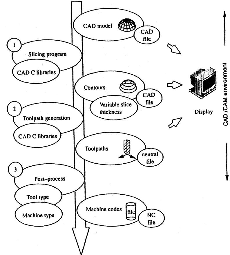
**Figure 4:** Details of process planning issues necessary in adaptive laminated machining (shown in the highlighted boxes in Figure 3).
