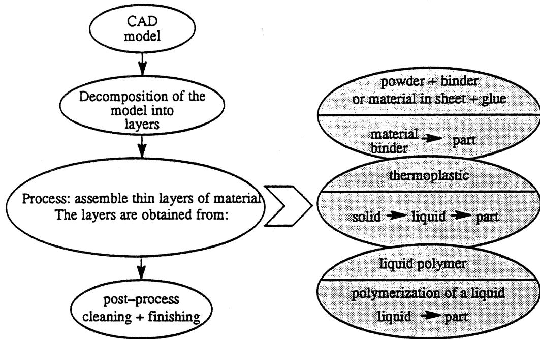
**Figure 1:** Overview of Free Form Fabrication
