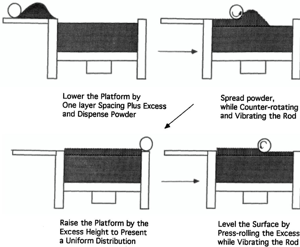
Figure 2. Press-rolling Sequence.
