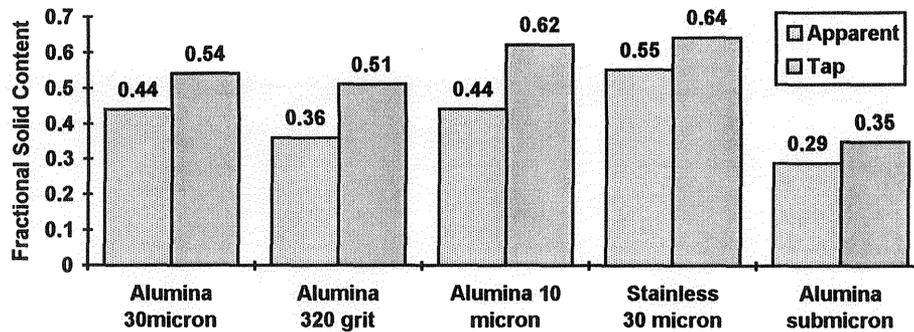
Figure 3. Apparent and tap densities of various powders
