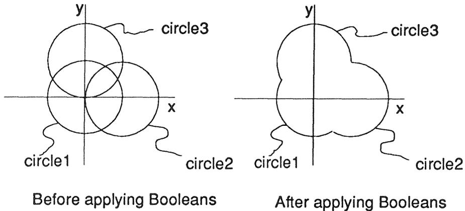
Figure 3. CSG slicing and set operations for SFF [7].
