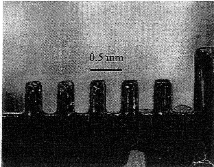
Fig. 3(B). The 2 pins/mm pattern in the T-PART build with Small Spot SLA
