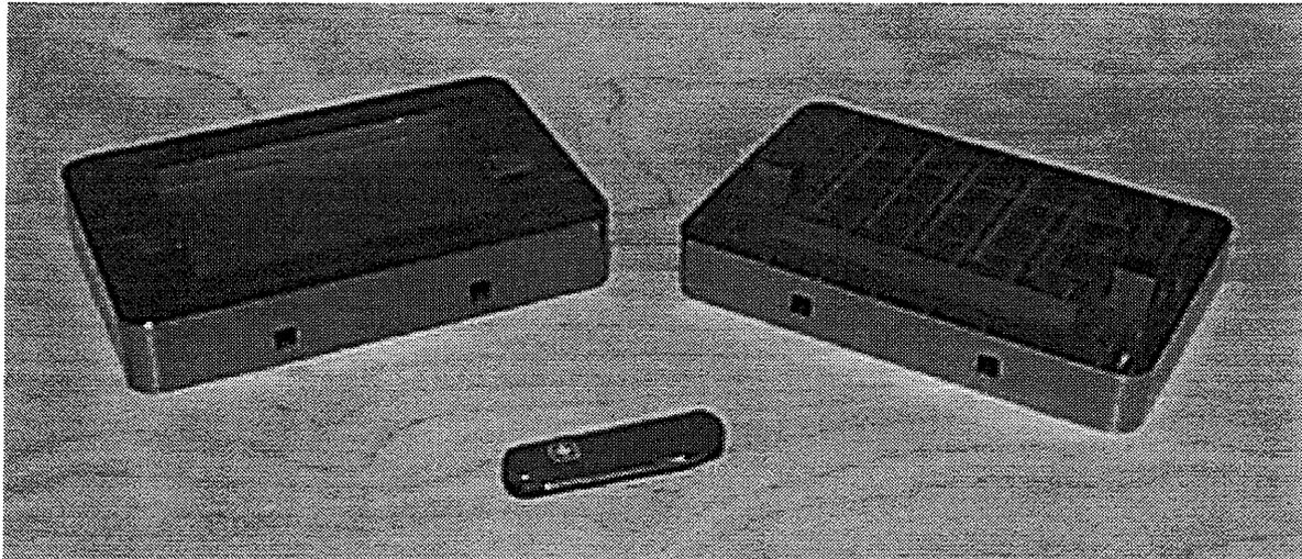
Figure 3: Photograph of injection molding tool made with laser system.
