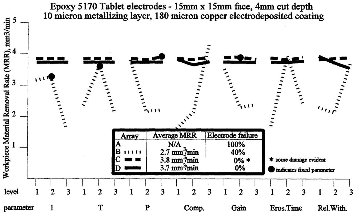
Figure 12 SL EDM electrode Material Removal Rate (MRR) optimization
