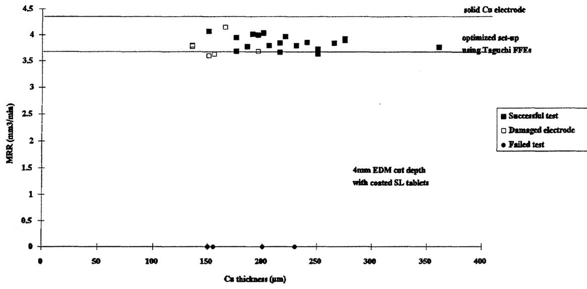
Figure 9 SL EDM electrode MRR versus copper thickness
