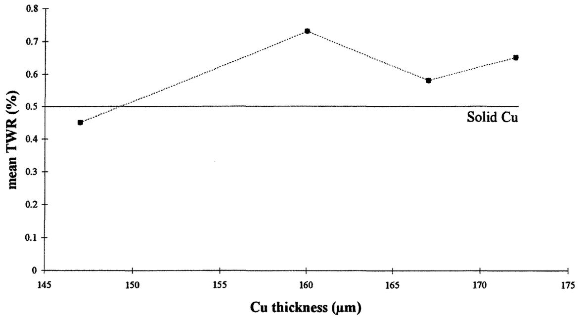
Figure 2 SL EDM electrode TWR versus copper thickness
