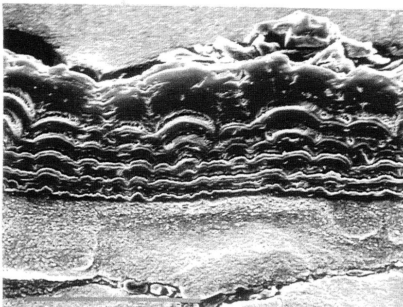
**Figure 4--SEM micrograph of 10 layer SiC SALD deposit**
