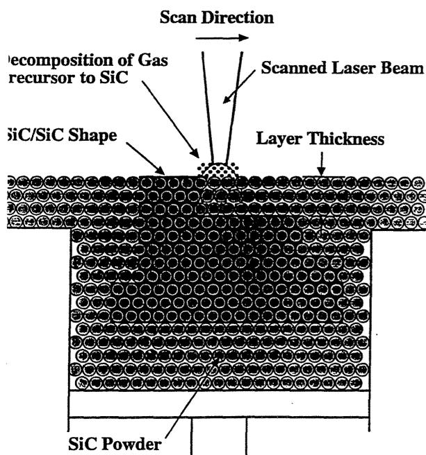
Figure 2--Schematic of SALD
