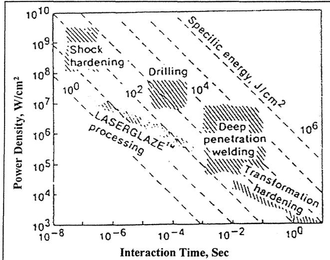
Fig. 1 Beam-material interaction spectrum<sup>2</sup>. A large number of commercial processes of surface material processing can be carried out at cw intensity levels from 1 kW/cm<sup>2</sup> to 1 MW/cm<sup>2</sup>.
