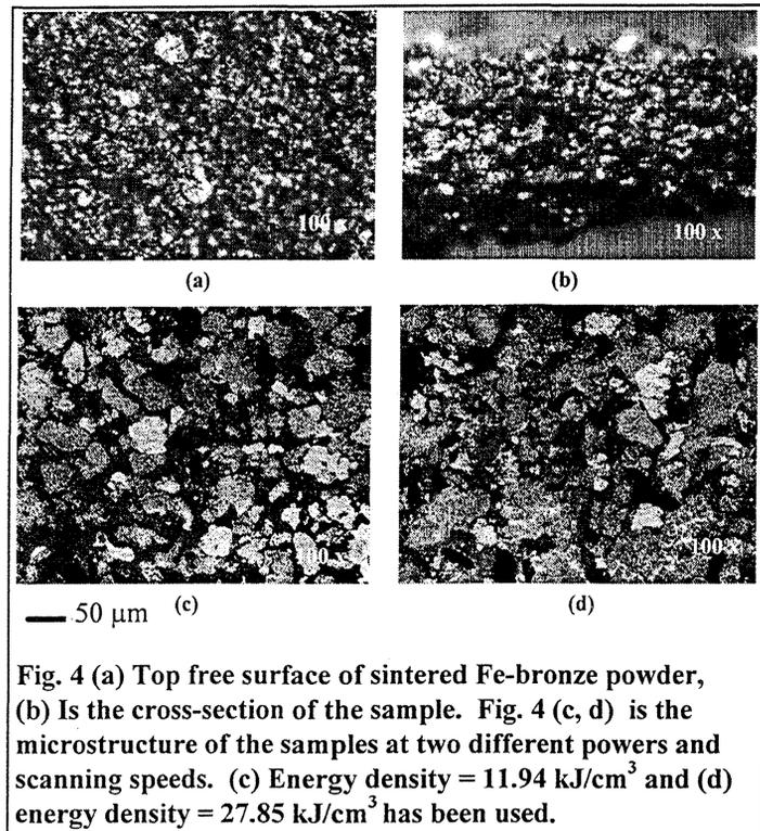
Fig. 4 (a) Top free surface of sintered Fe-bronze powder, (b) Is the cross-section of the sample. Fig. 4 (c, d) is the microstructure of the samples at two different powers and scanning speeds. (c) Energy density = 11.94 kJ/cm<sup>3</sup> and (d) energy density = 27.85 kJ/cm<sup>3</sup> has been used.
