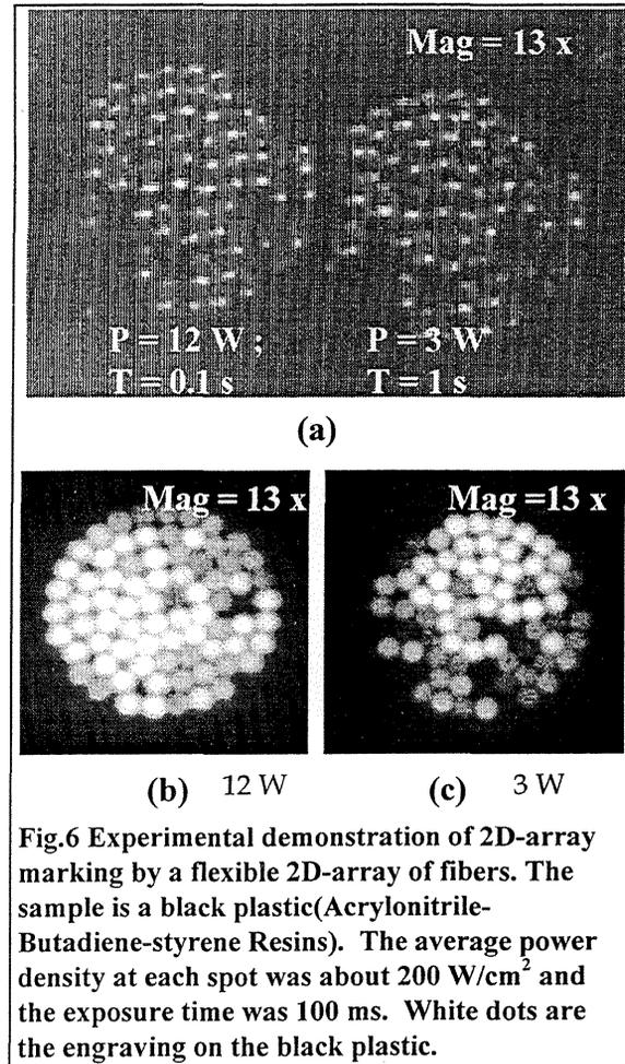
Fig.6 Experimental demonstration of 2D-array marking by a flexible 2D-array of fibers. The sample is a black plastic (Acrylonitrile-Butadiene-styrene Resins). The average power density at each spot was about  $200 \text{ W/cm}^2$  and the exposure time was 100 ms. White dots are the engraving on the black plastic.
