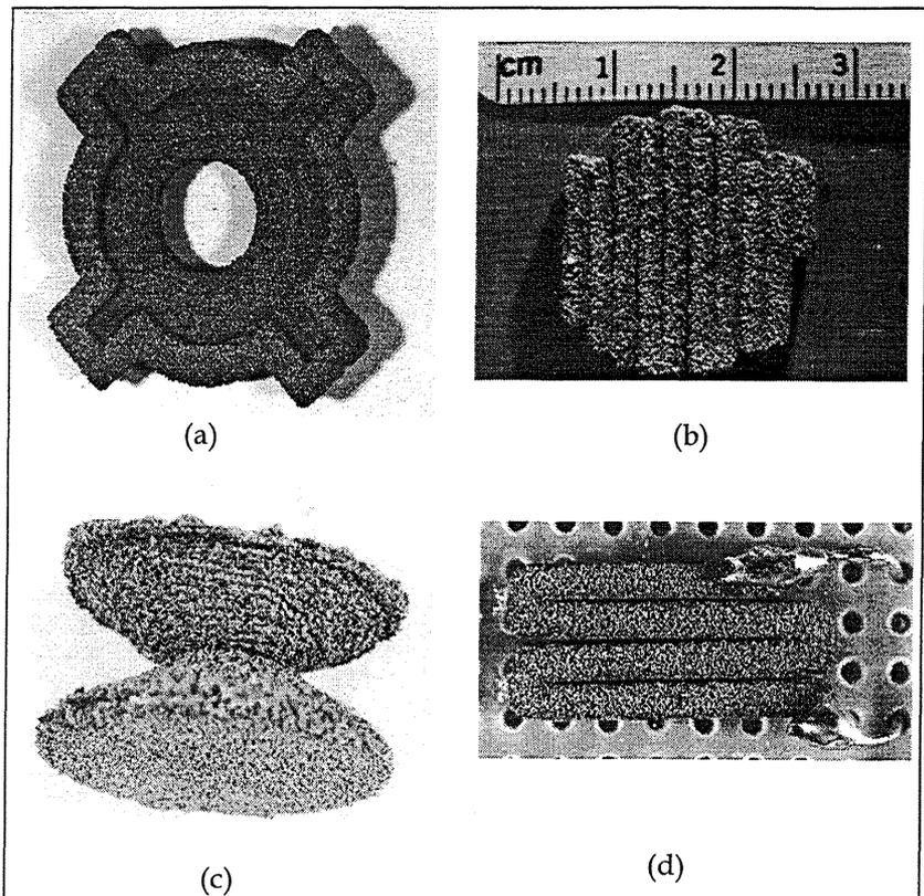
Fig. 3 (a-c) The sintered samples made from iron-bronze premix powder in an argon atmosphere.
