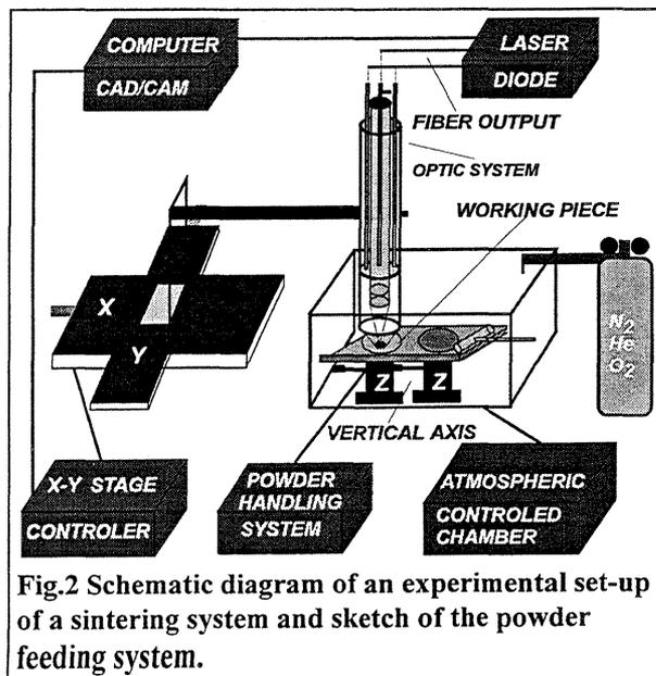
Fig.2 Schematic diagram of an experimental set-up of a sintering system and sketch of the powder feeding system.
