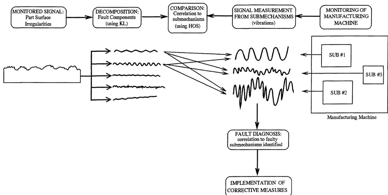
**Figure 1:** Feature Extraction and Fault Diagnosis Approach.
