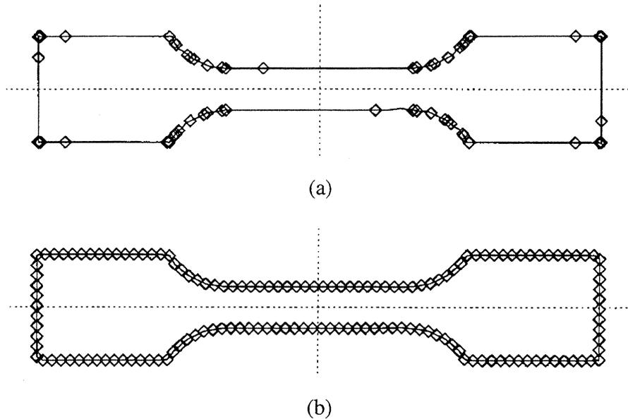
Figure 6. Cubic NURBS representation of the contour from Figure 3.
