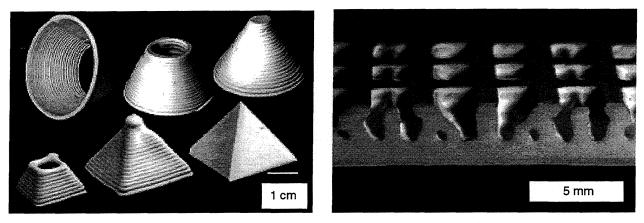
Figure 5 Examples of sintered aluminum oxide parts made by Robocasting: (A) Shows thin walled and solid parts. Notice that with minimal machining surfaces can be made smooth; (B) This cross section shows the symmetry and control that can be obtained in an intricate structure with tailored porosity. Due to regions with closed porosity and undercuts, this part could probably not be made by traditional molding or machining techniques.
