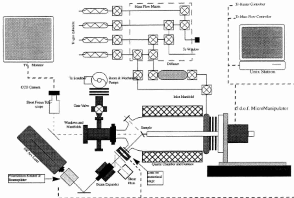
**FIGURE 1.** Schematic diagram of the 3-D LCVD reactor.
