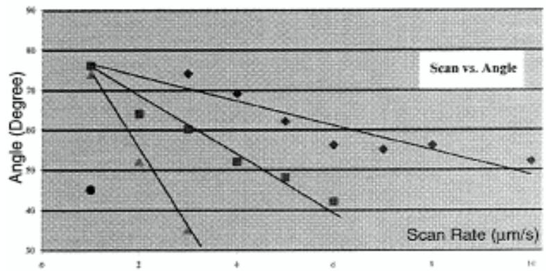
**FIGURE 3.** Rod angle with substrate as a function of scan rate for various precursor pressure. Laser power adjusted to maintain constant volumetric deposition rate. Deposit: carbon from ethylene. Substrate: quartz. Legend:
