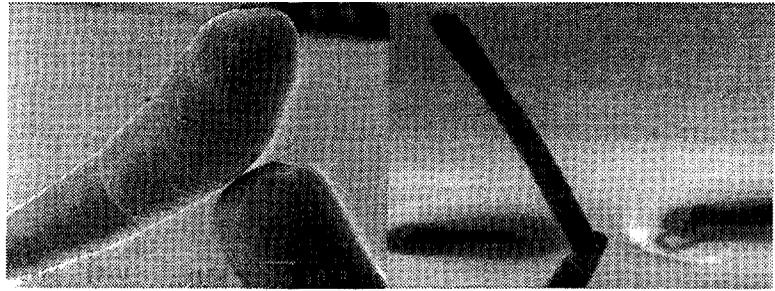
**FIGURE 7.** Typical joining problems with stationary laser growth. Left: First rod does not occult the laser and the rods grow past each other. Right: The first rod occults the laser and the second rod grows on top of the first one.
