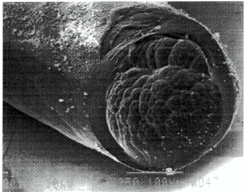
**FIGURE 6.** Close-up view of a fractured angled rod showing the uniform graphitic "skin", amorphous core, and axial ridge on the posterior side of the rod.
