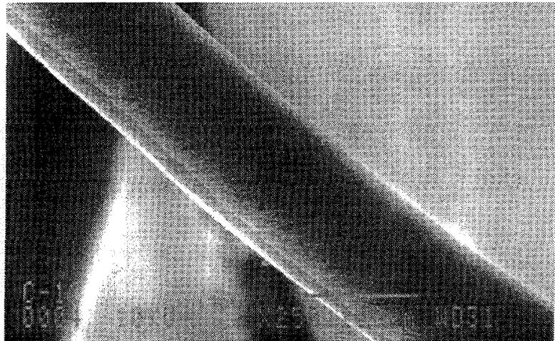
**FIGURE 5.** Close-up view of an angled rod showing the characteristic ridge on the posterior side.
