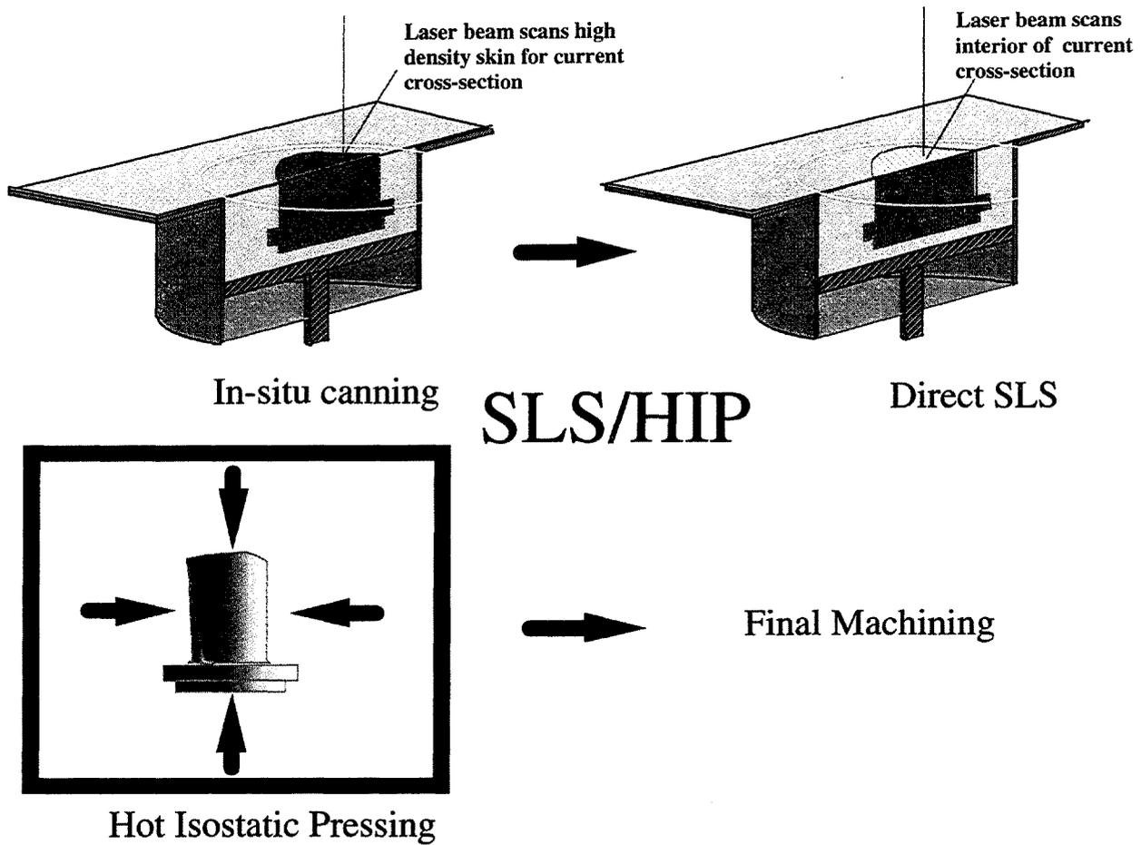
**Figure 1** The SLS/HIP Process
