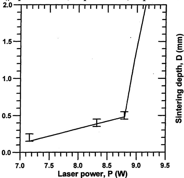
Figure 2. Effect of laser power on sintering depth. Powder mixture for chemical reaction (1). Laser scan velocity  $v = 25 \text{ cm/s}$ ,  $d = 50 \text{ mkm}$ .
