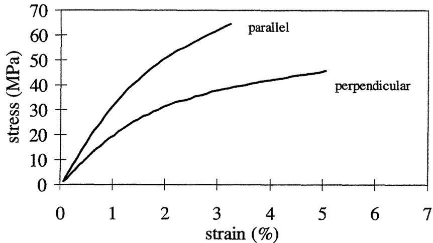
Figure 5. Typical tensile stress-strain curves for polymer N2 after UV postcure
