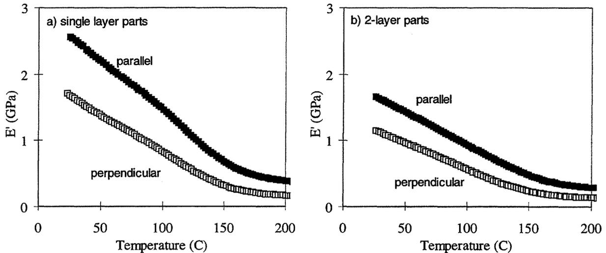
Figure 4. Anisotropic elastic modulus of N2 resins.
