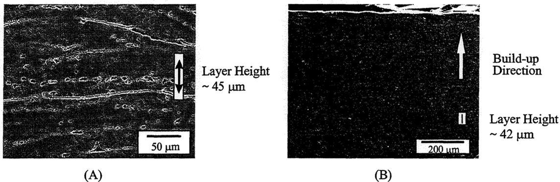
**Figure 6.** Cross sectional microstructures of sintered powder bed prepared with and without wetting agent in the slurry are shown in (A) and (B), respectively. Lamination defects are observed in (A) due to the wetting behavior of the slurry on binder printed regions.
