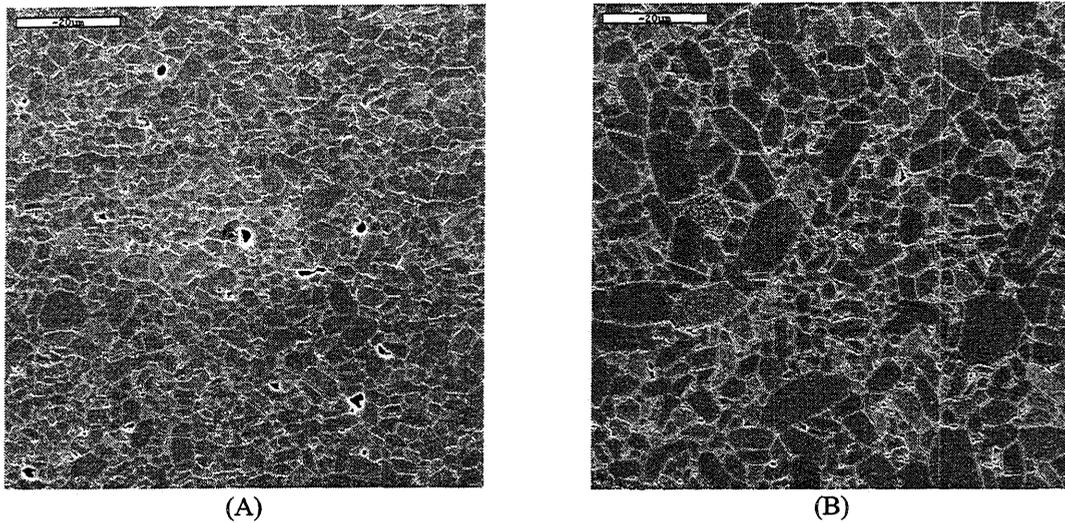
**Figure 2.** Polished cross-sections of samples sintered at 1650°C. Microstructure of slurry-based 3DP parts (A) are similar to powder beds prepared by slip casting (B). (Scale marker bar is 200  $\mu\text{m}$ ).
