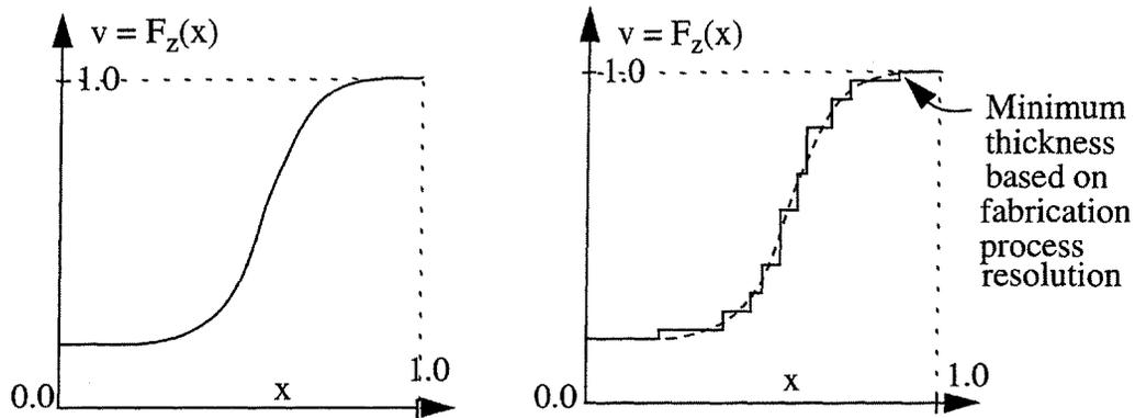
**FIGURE 6.** Approximation of a distribution function by series of step functions
