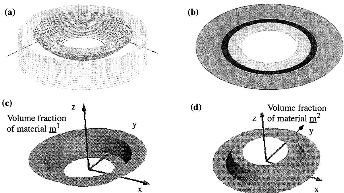
**FIGURE 7.** (a) Adaptive slicing (b) Material Distribution at slice  $z=0.8$  (c) Variation of volume fraction of material-1 in slice  $z=0.8$  (d) Variation of volume fraction of material-2 in slice  $z=0.8$
