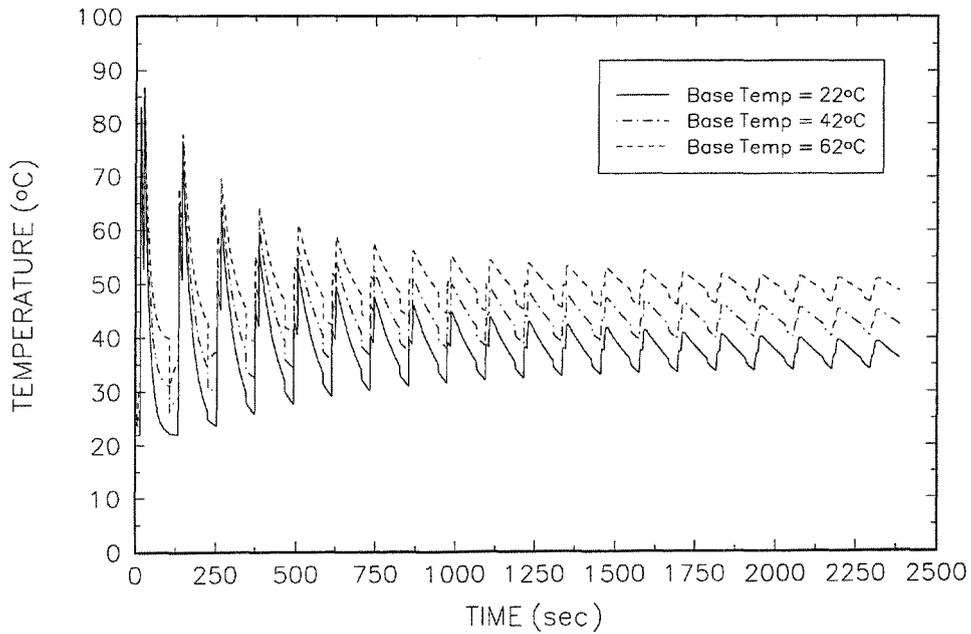
**Figure 6 :** predicted temperature profiles, analyzing effect of varying base plate temperature on overall part temperature.
