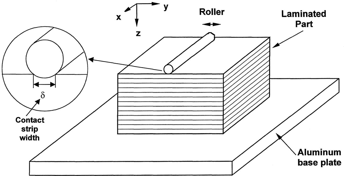
**Figure 2** : geometry and coordinate system for model.
