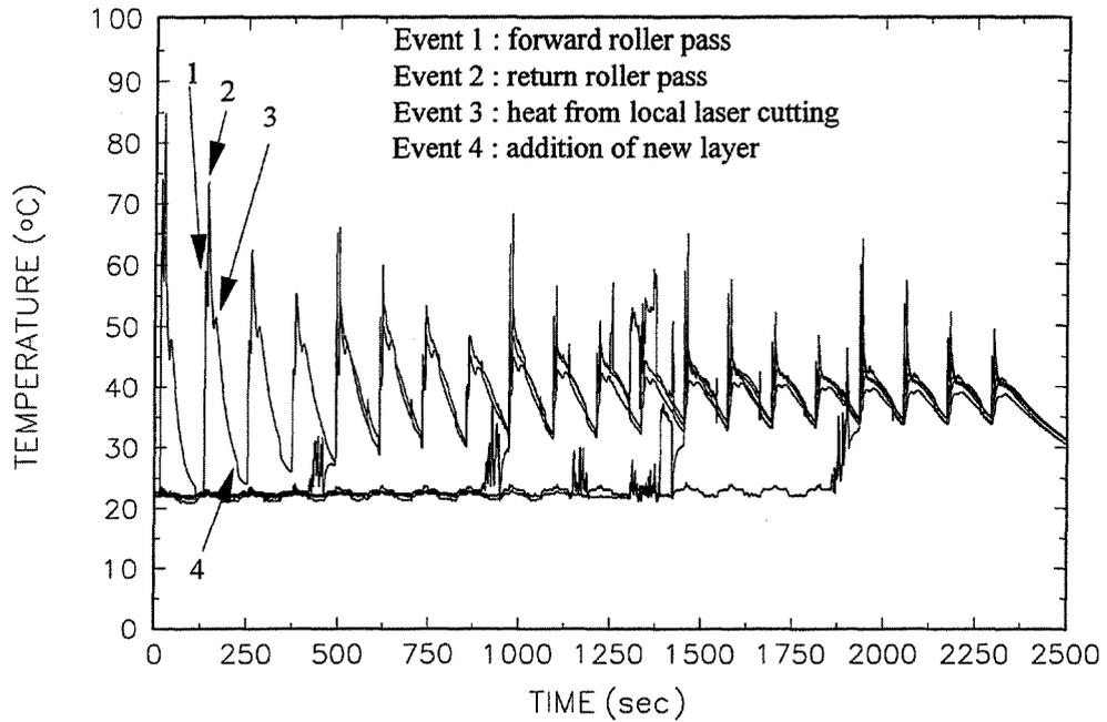
**Figure 3** : measured temperature profiles from embedded thermocouples above the 0<sup>th</sup>, 4<sup>th</sup>, 8<sup>th</sup>, 12<sup>th</sup>, and 16<sup>th</sup> layers in a 20 layer ceramic part built on a LOM2030.
