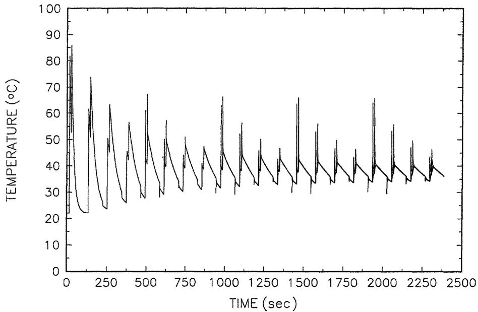
**Figure 4** : predicted temperature profiles for nodes above the 0<sup>th</sup>, 4<sup>th</sup>, 8<sup>th</sup>, 12<sup>th</sup>, and 16<sup>th</sup> layers in a 20 layer ceramic part.
