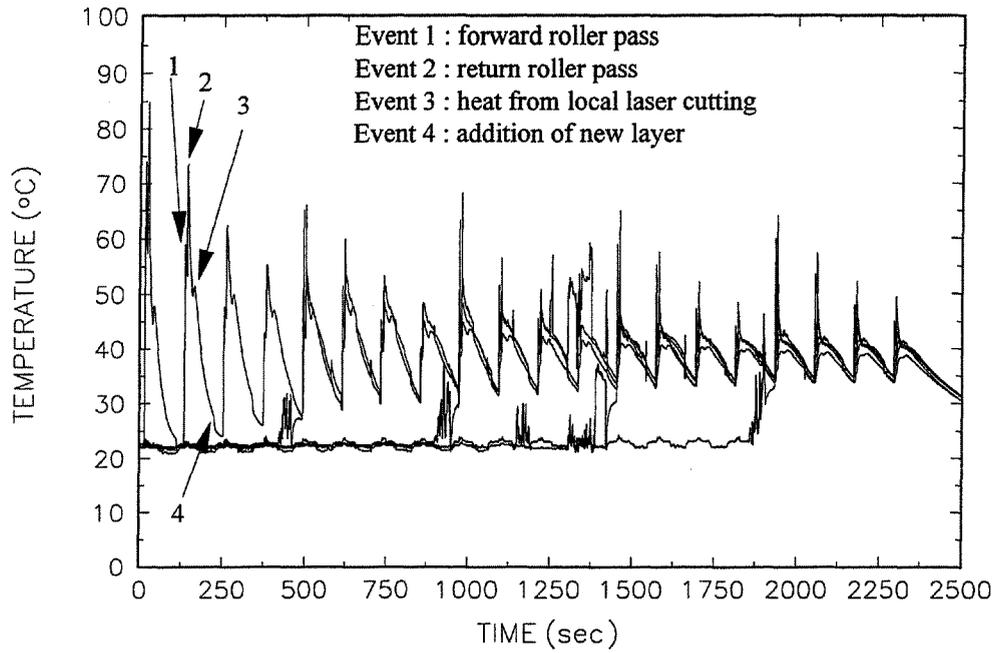
**Figure 3** : measured temperature profiles from embedded thermocouples above the 0<sup>th</sup>, 4<sup>th</sup>, 8<sup>th</sup>, 12<sup>th</sup>, and 16<sup>th</sup> layers in a 20 layer ceramic part built on a LOM2030.
