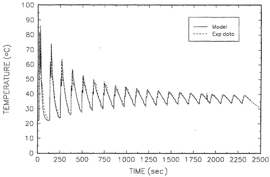
**Figure 5 :** measured and predicted temperature profile for thermocouple just above the 0<sup>th</sup> layer (foam tape base).
