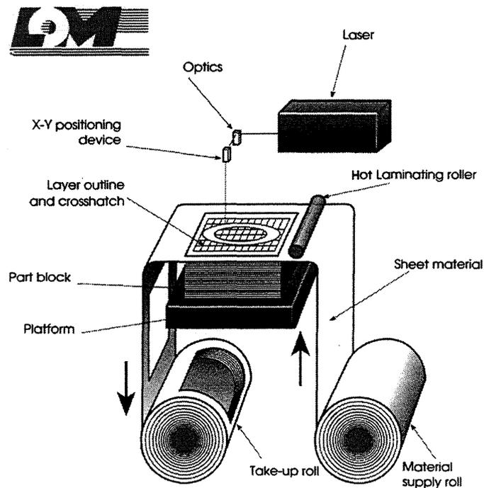
**Figure 1** : schematic of the LOM process.
