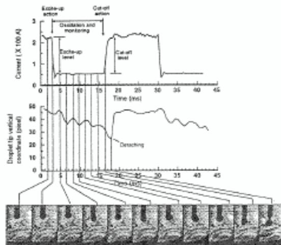
Fig. 4 Experimental observation of the excited droplet oscillation and detachment.
