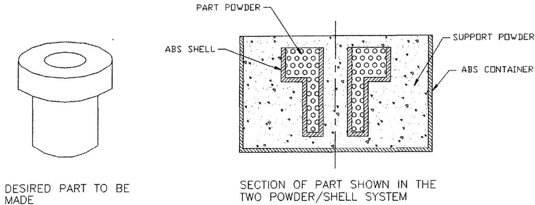
**Figure 2: Two Powder-Polymer Shell System**
