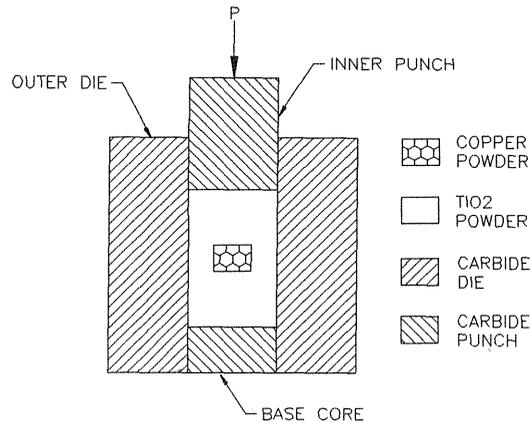
**Figure 3: Schematic of Experimental Setup**
