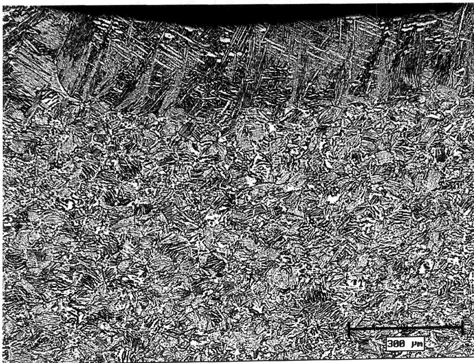
Figure 4. Can-core interface
