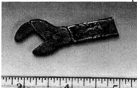
Fig.5 Sintered Wrench part, broken during the BBO
