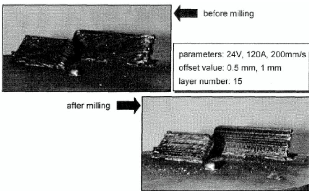
**Fig. 4:** Inclined walls with angles of 24° and 44°
