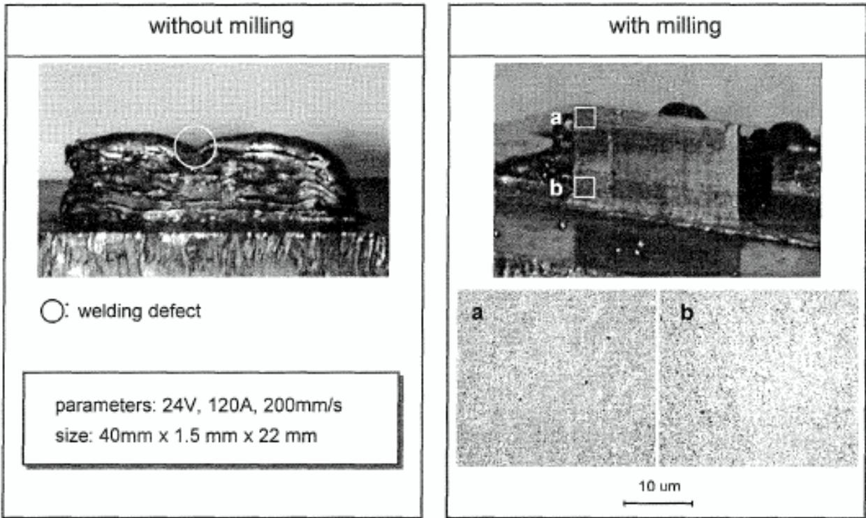
**Fig. 3:** Thin-walled parts without milling and with milling
