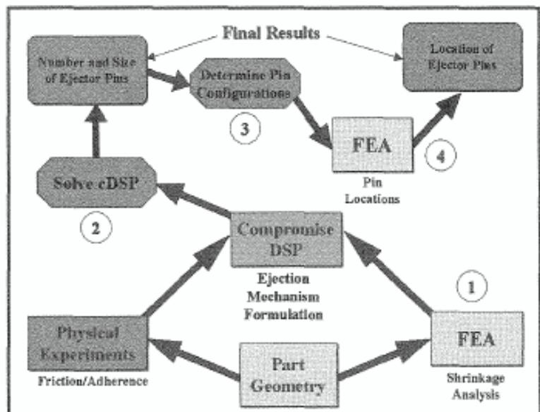
Figure 2 Process Flowchart
