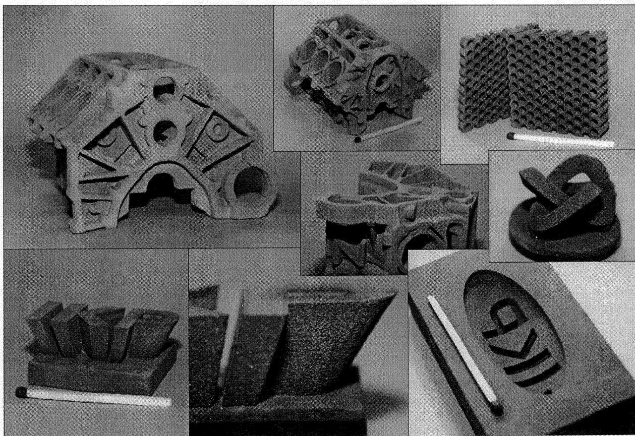
**Figure 9: Complex test samples with overhangs, under cuts and inner sections like moulds and combs**
