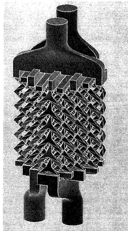
**Figure 12: Possible orientation of a liquid to liquid heat exchanger using TetraLattice. The two shaded regions represent the fluid within the heat exchanger (illustration by Adrian Sikorski).**
