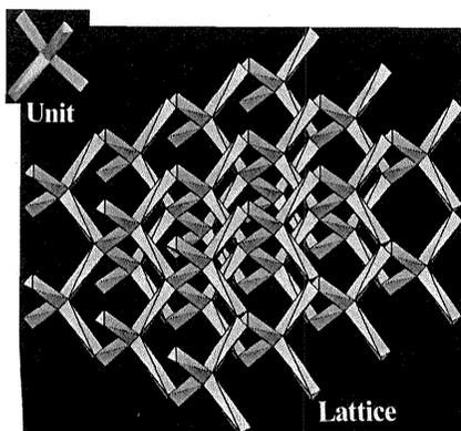
**Figure 1. TetraLattice structure with repeating unit shown**
