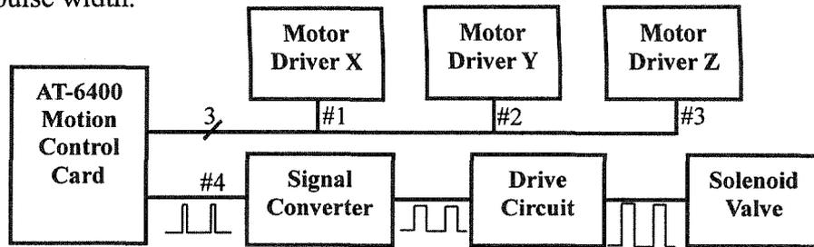
Figure 4. Schematics of the electronic control device
