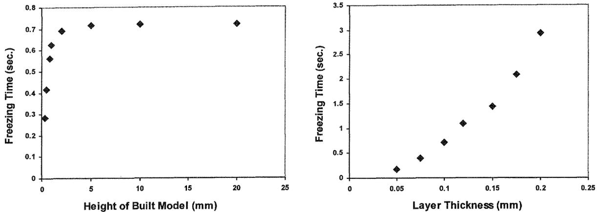
Figure 6. Influence of built model height and newly deposited layer thickness on freezing time
