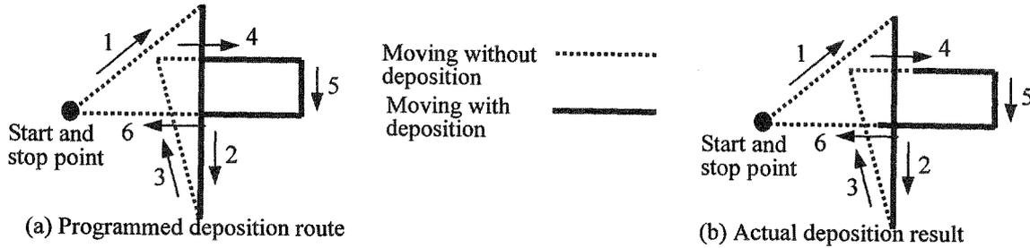
Figure 8. Drawing route to measure valve start-stop errors
