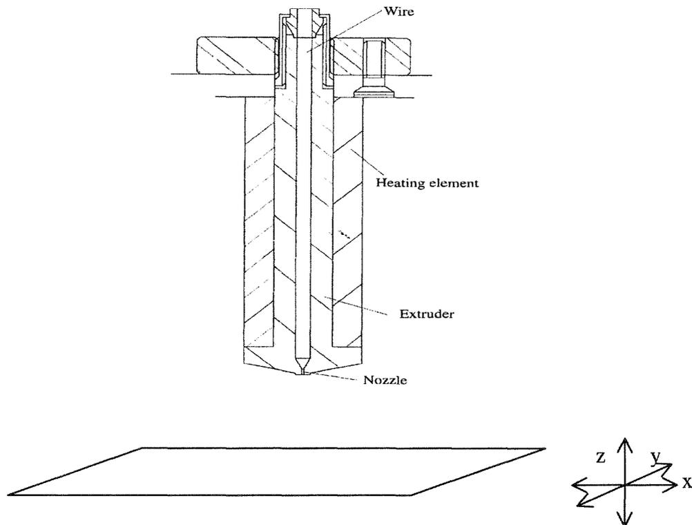
**Figure 2:** Extrusion head
