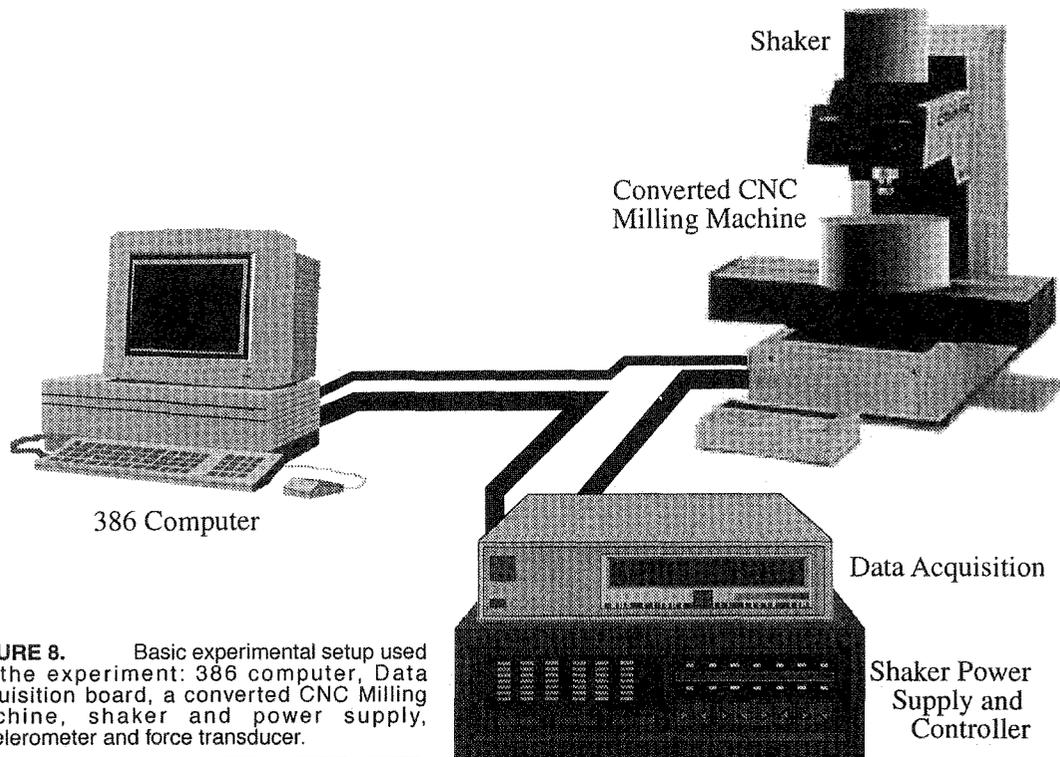
**FIGURE 8.** Basic experimental setup used for the experiment: 386 computer, Data acquisition board, a converted CNC Milling machine, shaker and power supply, accelerometer and force transducer.
