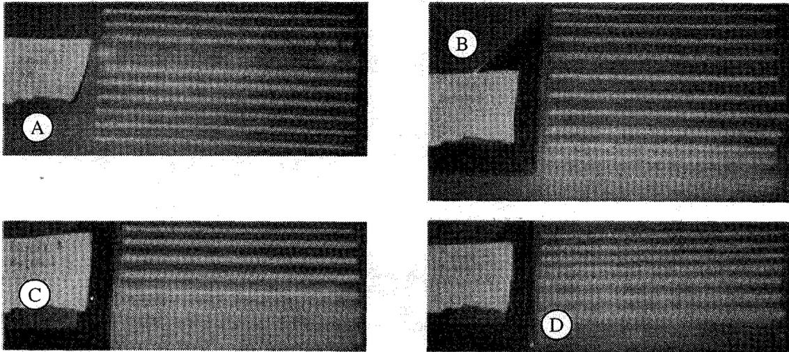
**FIGURE 19.** Sample deposition lines of  $\varnothing 220\mu$ m spherical glass beads on 120 grit sandpaper. Listed below are frequency and amplitudes, from top to bottom. Average position of the nozzle opening is 2-3mm above the substrate.
