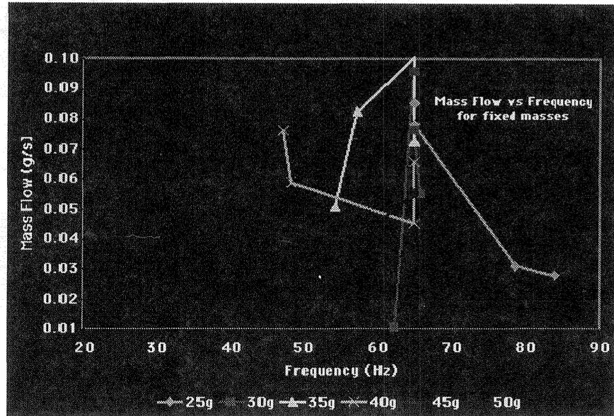
FIGURE 13. Mass flow vs. frequency characteristics interpolated for fixed hopper masses (but varying amplitudes).
