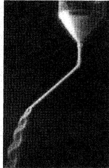
**FIGURE 16.** In-phase stroboscopic view of the powder flow through a downcomer at 45°.
