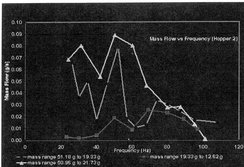
FIGURE 11. Sample mass flow rates vs. frequency plots for series of runs through variable hopper masses.
