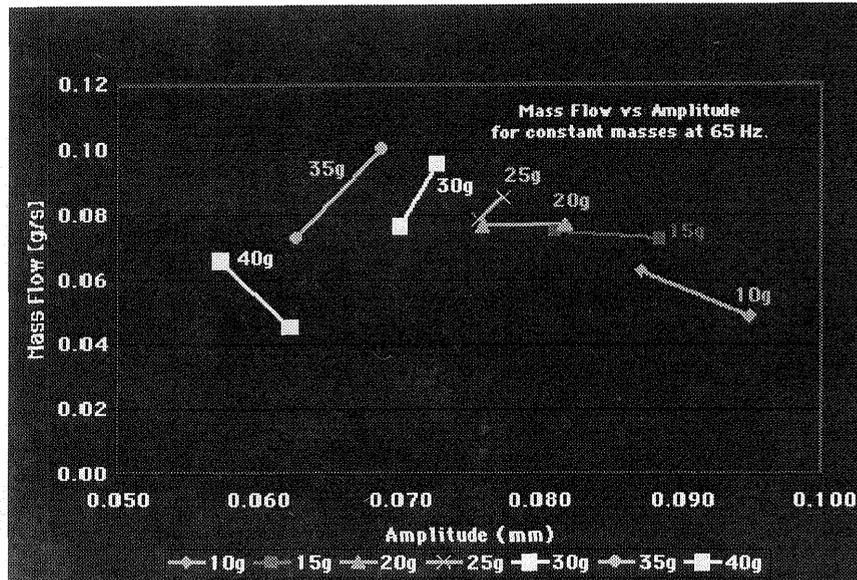
FIGURE 15. Composite of the mass flowrate vs. amplitude derived from Figures 11-14 for fixed hopper masses of 10, 15, 20, 25, 30, 35, and 40 grams, and fixed frequency of 65 Hertz.
