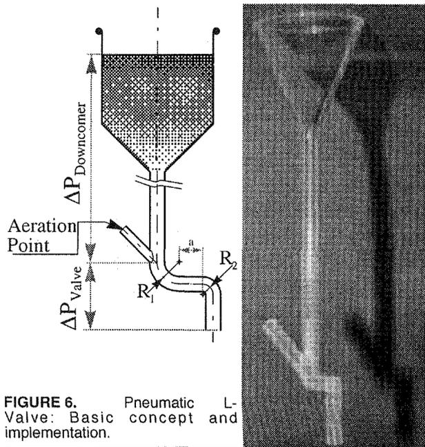
**FIGURE 6.** Pneumatic L-Valve: Basic concept and implementation.
