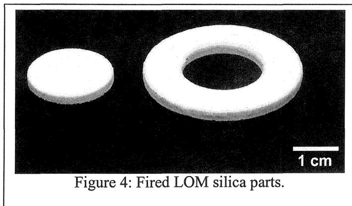
simple parts by the LOM process. Simple LOM green silica parts were used to establish suitable binder burn out schedules. Following successful binder burn out, the samples were subjected to firing at temperatures of 1100°C and 1300°C for 2 to 6 hours, Figure 4. The fired part density ranged between 70% and 80% of theoretical density of fused silica (2.2 g/cc). Associated firing shrinkage was 1% - 3% in X and Y and 3%-5% in Z.
