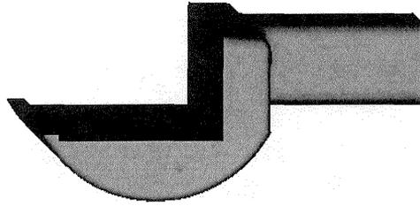
This part has been designed to test the susceptibility of the shell to failure when there is a point of high stress on the piece. The thin, sharp front edge of the piece is an area where shell fracture during burnout is much more likely to occur than for right angles or rounded surfaces. With this geometry it is efficient to compare the effect of the casting, autoclaving and burnout process on the type of resin or to compare different processing methods with the same material.
