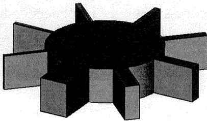
Several test parts have been designed to evaluate these properties. One is a disc with radiating arms of varying thickness. The objective of this piece is to see how thin a section can be before there is insufficient drainage of resin from the section. In addition, if the arm is too susceptible to bending there may be deformation from the desired geometry during the casting process.
