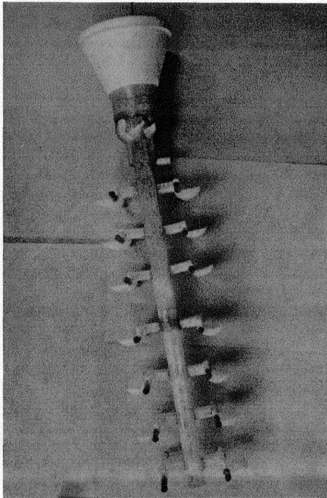
It is possible to build the casting tree with stereolithography instead of using the traditional wax tree (C.S. McDowell, M.C. Boomer, "Design of Stereolithography Trees for Use in the Investment Casting of Stereolithography Patterns"). This technique has the advantage of reducing the fracture of ceramic shells due to thermal expansion of the wax tree. Gates and runners can also be designed and built using stereolithography.
