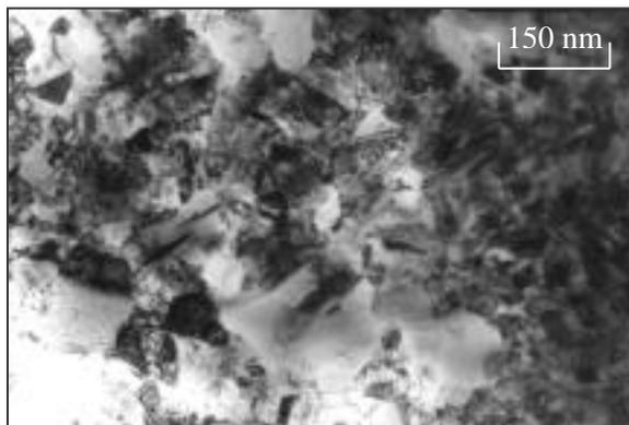
Fig.6. Microstructure of electroplated Ni (TEM)
