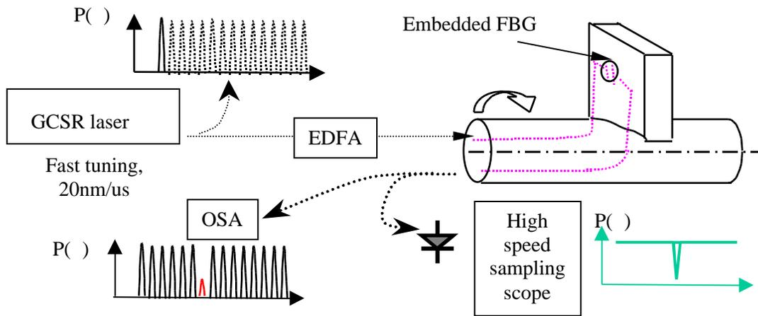
Fig.9. Remote sensing system for rotating parts with embedded fiber optical sensors
