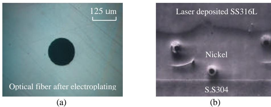
Fig.5. Embedded Optical fiber with good bonding
