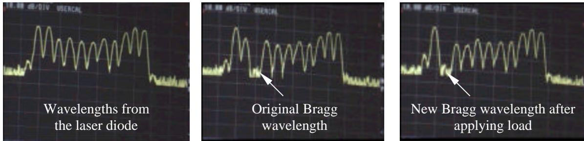
Fig. 11. Bragg wavelength shifts on OSA for the rotating part
