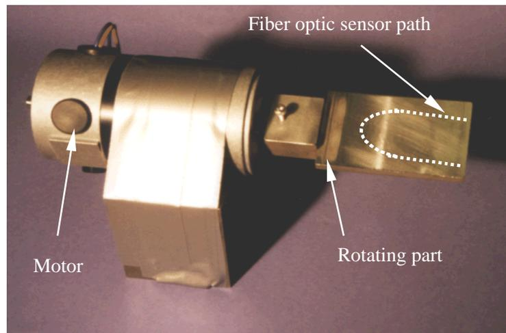
Fig.10. Rotating part with embedded fiber optic sensor
