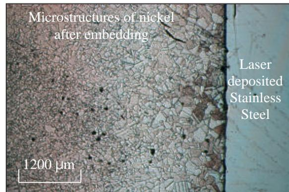
Fig.7. Microstructure of electroplated Ni after embedding
