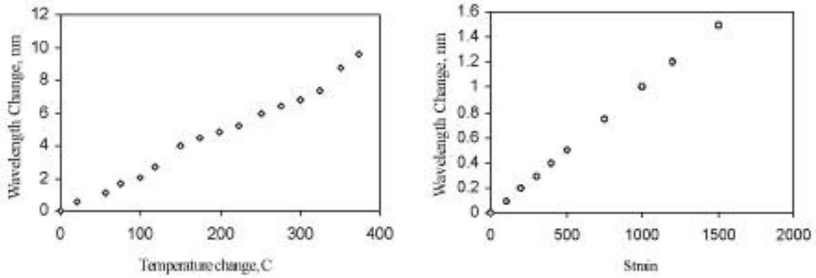
Fig.8. Experimental results for embedded FBG
