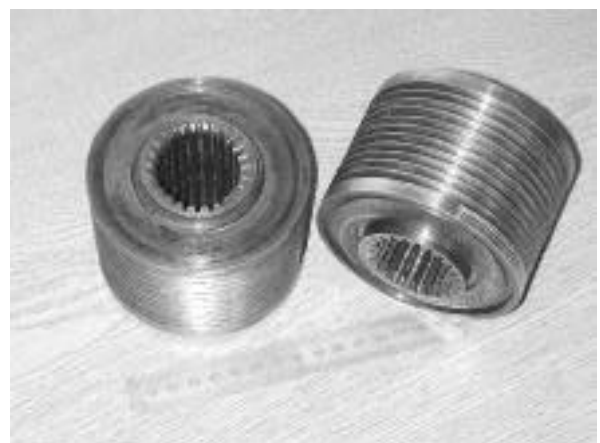
Figure 8. Two coolers after final machining.
