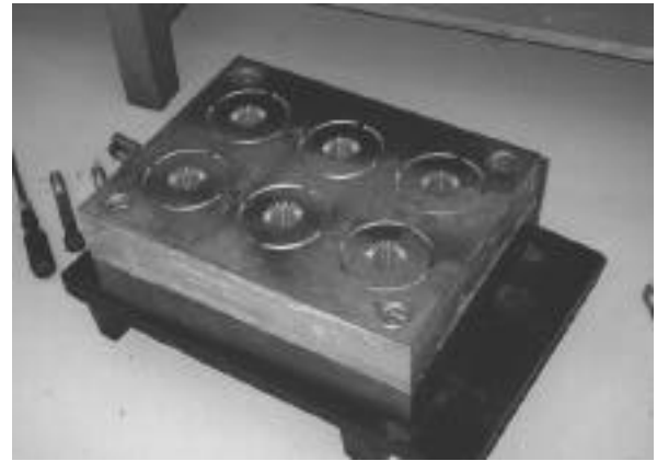
Figure 6. After heat treatment and removal of the top plate of the pressure jig.
