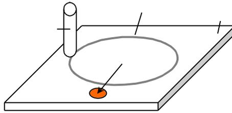
Fig. 4 The sketch of preheating temperature sensing
