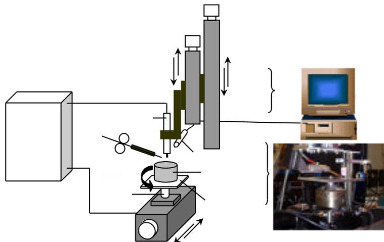
Fig. 1 The schematic diagram of the experiment system
