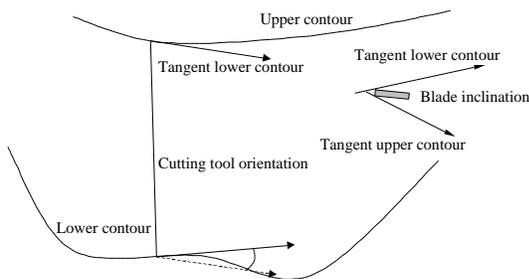
Figure 10 Yaw fixture from tangent calculation at both contours.
