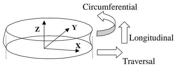
Figure 3. Principles of cutter movement along foam slab.
