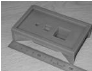
Figure 1. Wax master pattern built on 3D Systems ThermoJet
