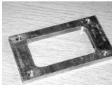
Figure 2. Machined copper frame for EDM tool holder attachment
