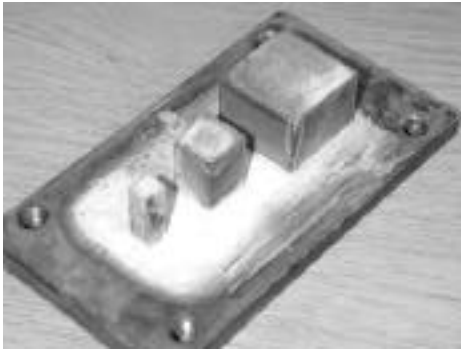
Figure 8. Final electroform – deep cavity S series, showing the three sizes of blocks
