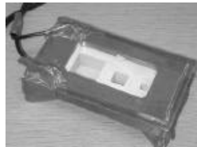
Figure 3. Sprayed master pattern with copper frame inserted and tape masking
