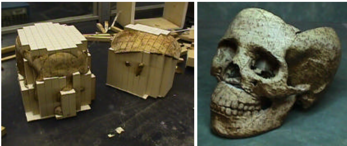
Figure 3. (left) LOM model before decubing. (right) Finished model.
