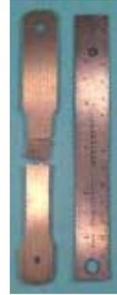
Figure 10: Tensile properties for infiltrated and cast specimens of the Ni – 4wt% Si. Image at right shows the infiltrated tensile specimen after failure.
