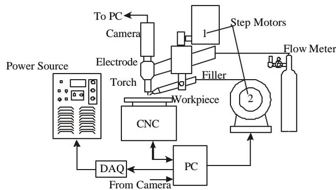
Fig. 2 Experimental set-up for GTAW
