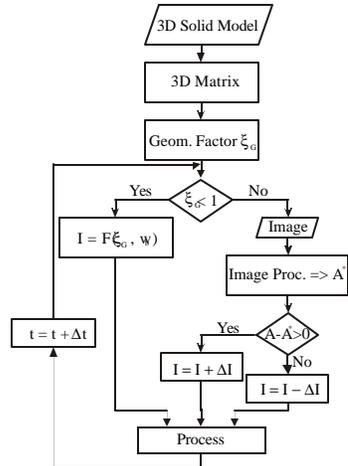
Fig. 8 Information flow in the designed controller
