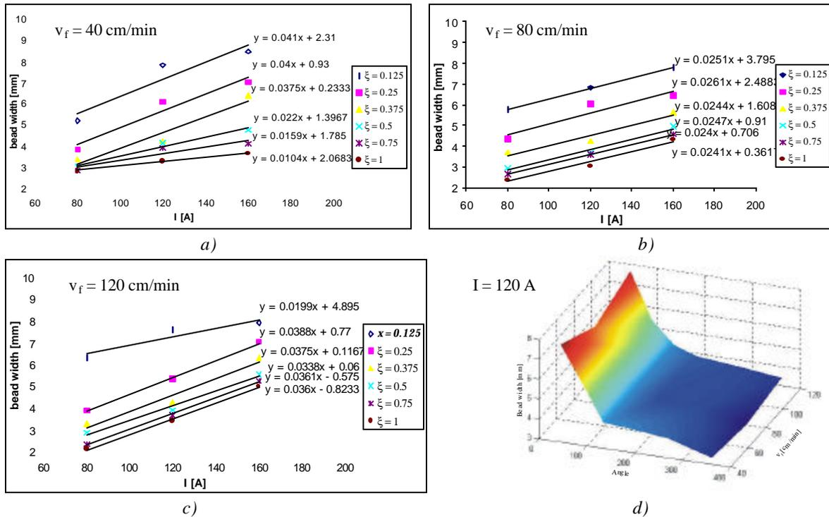
Fig. 5a, b, c and d – Influence of the geometry on the bead width. a, b, and c shows the bead width vs. current for three different wire feed speeds and for six different bead locations, d shows the change of the bead width when the wire feeding speed and heat sink are changed
