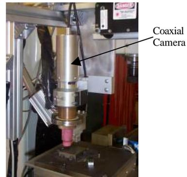
Fig. 3 Coaxially integrated camera with torch
