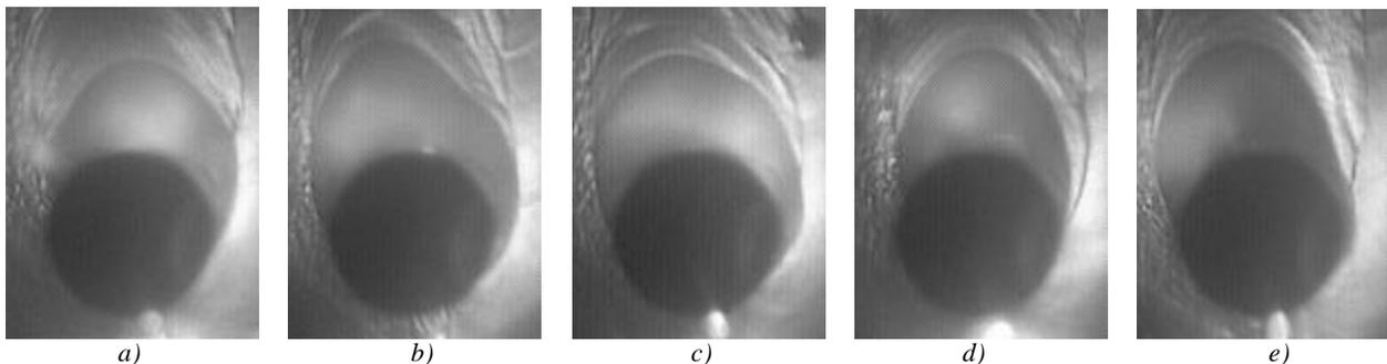
Fig. 7 Images of the fluctuating molten pool obtained for the same welding parameters
