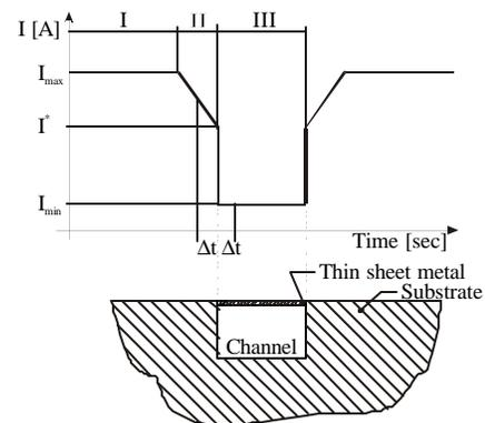
Fig. 6 Current vs. time is related to the part geometry
