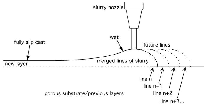
**Figure 4:** Schematic diagram of line merging concept
