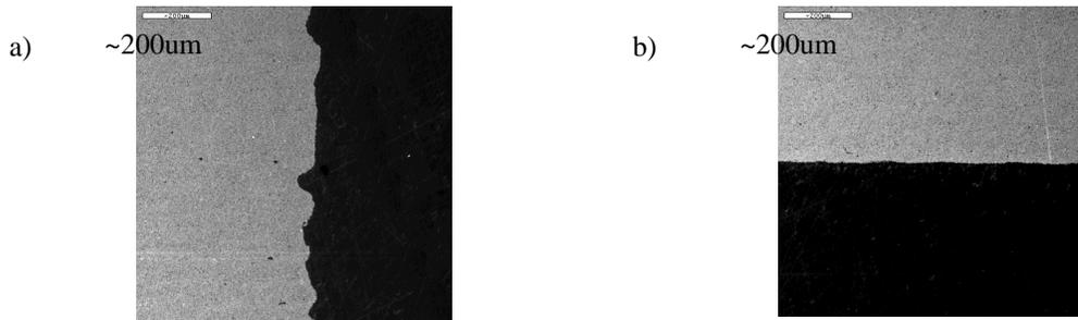
**Figures 8:** Images showing a) sidewall and b) bottom surface roughness. Images are of S-3DP<sup>TM</sup> MR2 components.
