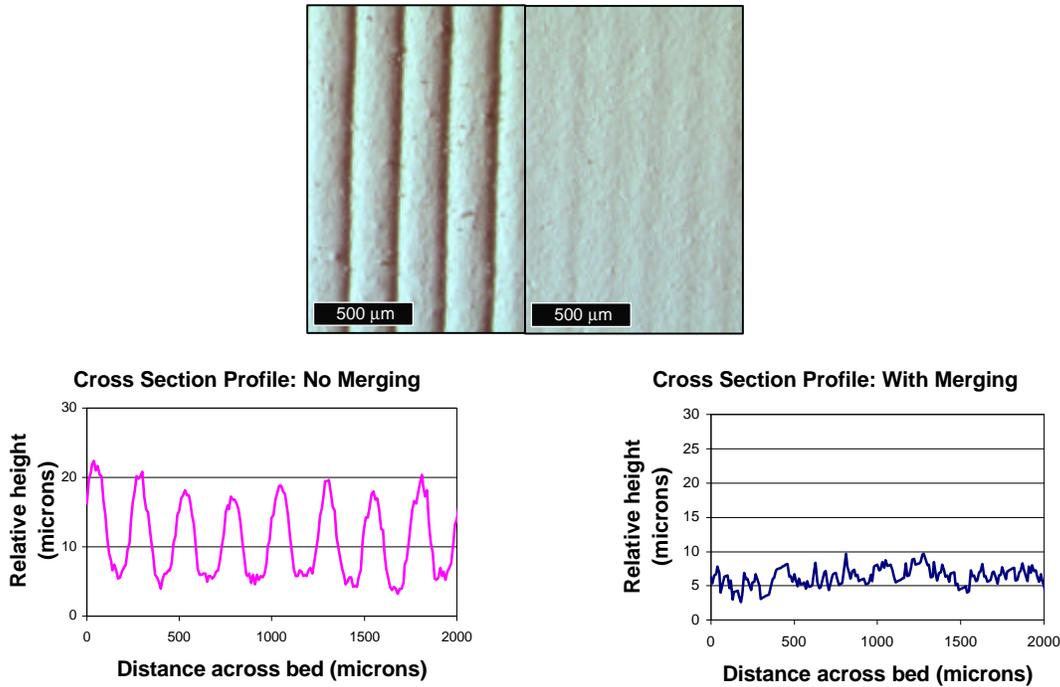
**Figure 6:** Top: Image of conventional (left) and merged (right) alumina powderbed. Bottom: Profilometry measurement of conventional (left) and merged (right) bed.
