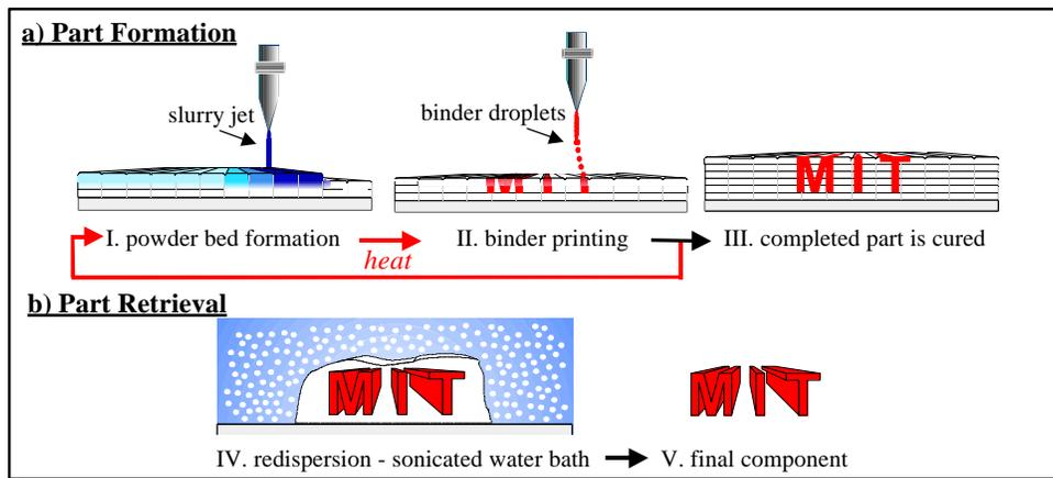
**Figure 2: Schematic of the Slurry-Based 3DP<sup>TM</sup> (S-3DP<sup>TM</sup>) Process.**
