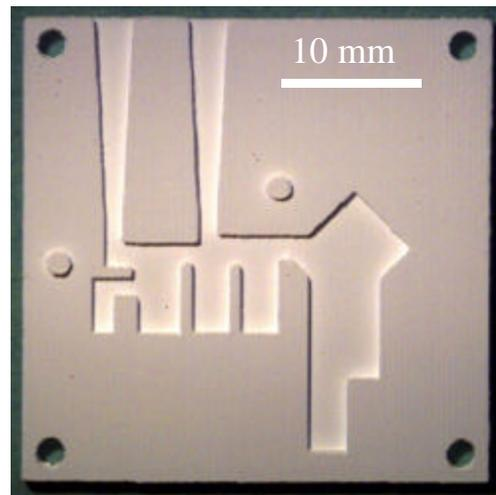
**Figure 11:** SEM cross section image of the S-3DP™ RF filter      **Figure 12:** Green S-3DP™ mm wave package
