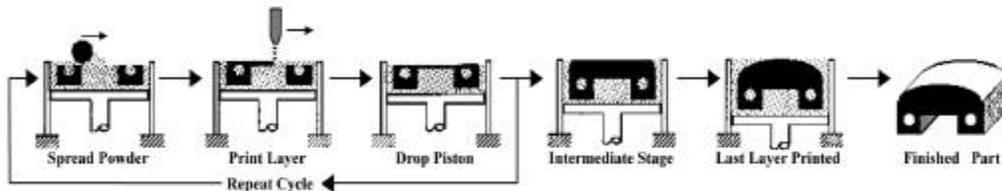
**Figure 1:** Schematic of the traditional (dry-powder) 3DP<sup>TM</sup> process.
