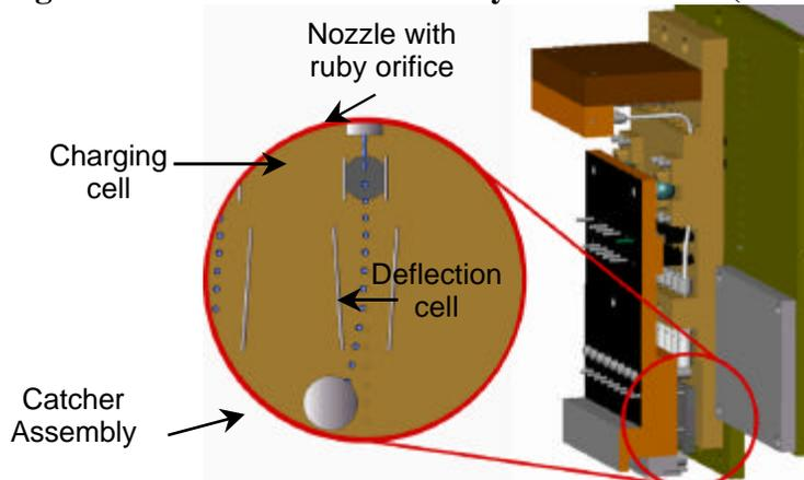
**Figure 3: Schematic of continuous jet print-head turned “Off”**
