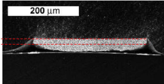
**Figure 7:** Cross section of binder primitive formed with CJ printing in an alumina powderbed. Hatched lines show proportion of layer height to binder primitive to reduce sidewall roughness.
