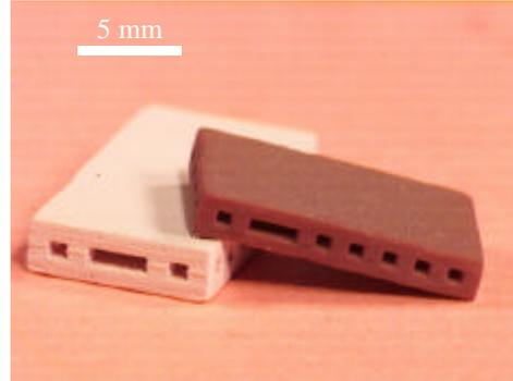
**Figure 16:** Green and dense BaTiO<sub>3</sub>-based EBG devices
