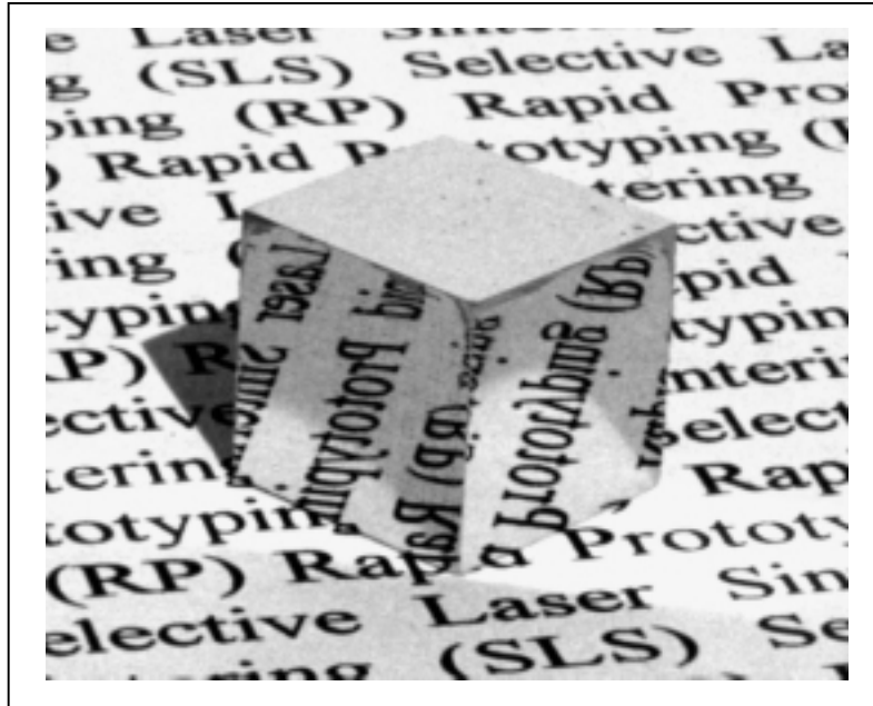
Figure 8: Stainless Steel 316L Cube Produced by DMLR (Density >99%)
