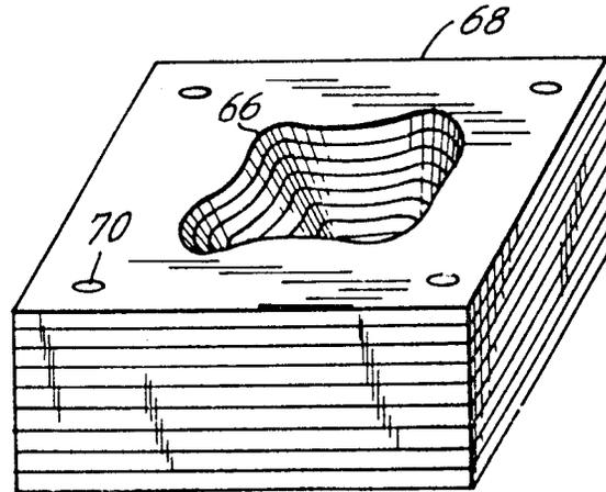
**Figure 2: Layered mold by DiMatteo (1974).**
