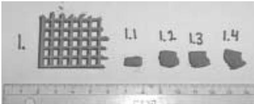
**Fig. 6.** Metallic bonded green bodies. Test 1. 1; Fill laser power: 35W, fill scan speed:500. 1.1; Fill laser power: 25W, fill scan speed:450. 1.2; Fill laser power: 30, fill scan speed:450 1.3; Fill laser power: 32.5W, fill scan speed:450. 1.4; Fill laser power: 35W, fill scan speed:450. Outline laser power:25W, outline scan speed 600, for all.
