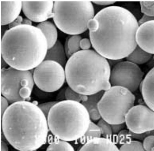
**Fig.2.** Anval2205. A stainless steel material, with the characteristic spherical shape of gas atomized metal powder. This alloy has been selected in order to maintain some desirable properties, should it reach full density after sintering. Size analysis: ASTM-E11 sieve, 91 % <  $-45\ \mu\text{m}$
