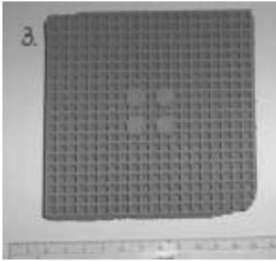
**Fig. 8.** Test 3. Laser power variation 32-40W and scan speed 300-400. Some initial curling and adherent movement during application of new layers. Small difference between parts, though a tendency to curl and brake out of position for pieces exposed to higher laser energy. Stable enough to be rinsed and handled in one piece.
