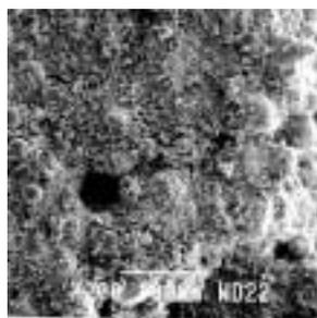
**Fig. 11.** Test 2. Green body surface of support mesh, laser power 35w scan speed 400.
