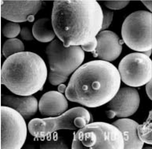
**Fig.1.** Anval9044. An alloyed tool steel material, with the characteristic spherical shape of gas atomized metal powder. The spherical shape is known to have the lowest interparticle friction and thus the best possible flowing behavior and packing. Size analysis: ASTM-E11 sieve, 88 % <  $-45\ \mu\text{m}$ .
