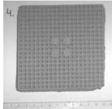
**Fig. 9.** Test 4. Laser power variation 30-40W and scan speed 250-350 Displays a similar behavior as in Test 3 (**Fig. 8.**) Though stronger green bodies, the tendency for curling shifting and for pieces to brake out of position is more obvious.
