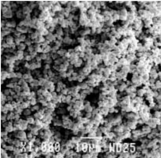
**Fig.4.** Carbonyl Iron SM: almost pure iron, with the spherical shape typical of carbonyl metal powder. In this size range (2-8  $\mu\text{m}$ ), the interparticle friction is associated with van der Waal's and electrostatic forces, and is thus increasingly independent of particle shape. Nevertheless, the spherical shape still is the best possible considering the achievable packing properties.
