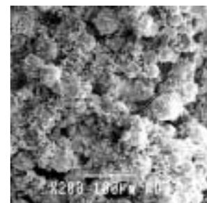
**Fig. 12.** Test 4. Green body of support mesh, laser power 40w scan speed 350.
