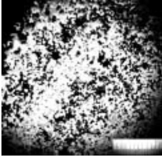
**Fig. 17.** Anval 2205, part 1.2, top view slightly angled to building direction. Slightly etched in 1 part ferric chloride, 10 parts hydrochloric acid & 20 parts water. Scale: 1 unit = 0.01 mm. Notice how the porosity has been positioned in between the layers.
